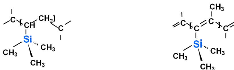
Figure 3. Chemical structure of PVTMS (left hand side) and of PTMSP (right hand side)
