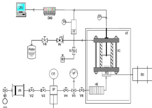
**Figure 1.** Schematic diagram of the apparatus. PS: Pressurized source; VP: volumetric press; SP: syringe pump; CB: cryostat bath; VP: vacuum pump; HE: heat exchanger; EM: electric motor; MS: magnetic stirrer; VC: view cell; AT: air thermostat bath (oven); TP: platinum resistance temperature probe; PT: pressure transducer; TR: temperature regulator; BD: bursting disc; FV: flow regulation valve; DAS: data acquisition system; CPU: central processor unit; V: valve.
