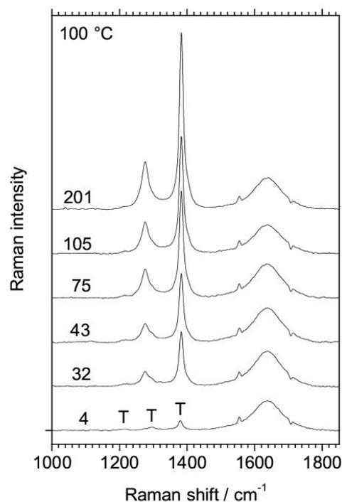
Fig. 2: Raman spectra of dissolved CO<sub>2</sub> in water at various pressures (bar) at 100 °C. T: Teflon. The peak at 1555 cm<sup>-1</sup> comes from atmospheric O<sub>2</sub> trapped in the probe. The spectra are offset for clarity.
