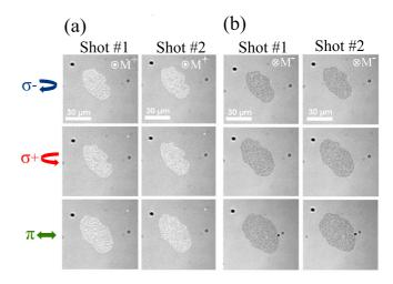
FIG. 6. (a) and (b) Magneto-optical Faraday images of a TbCo alloy film, with initial magnetization saturation up and down, illuminated with two consecutive pulses with three different polarizations and with an energy per pulse of 19 mJ/cm<sup>2</sup>. Each of the two laser pulses induces thermal demagnetization of the irradiated area. The white (dark) contrast in (a) [(b)] corresponds to a reversal to down (to up).
