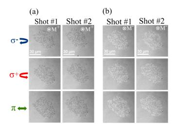
FIG. 3. (a) and (b) Magneto-optical Faraday images of a Pt (4.5 nm)/Co (0.6 nm)/Pt (4.5 nm) continuous film, with initial magnetization saturation up and down, illuminated with two consecutive pulses with three different polarizations and with an energy per pulse of 14 mJ/cm<sup>2</sup>. Each of the two laser pulses induces thermal demagnetization of the irradiated area. The dark (white) contrast in (a) [(b)] corresponds to a reversal to down (to up).
