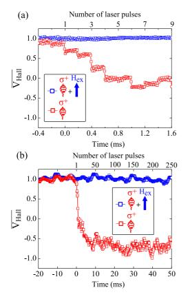
FIG. 5. (a) and (b) Time evolution of the anomalous Hall voltage of a 5- $\mu$ m-wide Pt (4.5 nm)/Co (0.6 nm)/Pt (4.5 nm) Hall cross initially saturated up, under the action of a 35-fs laser beam with a 5 kHz repetition rate and a laser fluence of 10 mJ/cm<sup>2</sup>, with (blue curve) and without (red curve) adding a small external magnetic field  $H_{ex}$  of 20 mT. The corresponding number of laser pulses is shown in the upper row.
