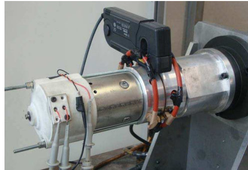
Figure 16. Prototype with slip rings for internal measurements.
