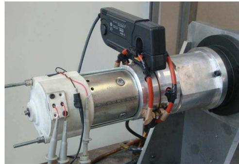
**Figure 16.** Prototype with slip rings for internal measurements.
