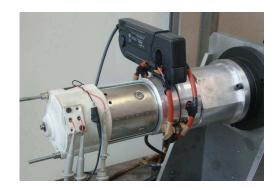
Figure 16. Prototype with slip rings for internal measurements.
