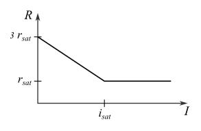
Figure 20. Non-linear electrical contact model.
