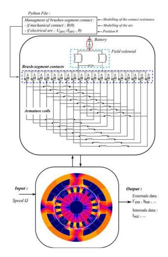
Figure 11. Description of algorithm with magnetic/electric coupling.
