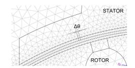
Figure 13. Description of the mesh in the air gap.
