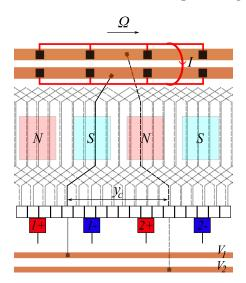
Figure 15. Principle of measurement of the internal waveforms.
