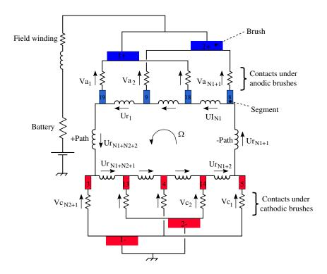
Figure 4. Equivalent electrical circuit of the armature represented in Figure 1 for the specific position of the brushes on the commutator represented on Figure 2 (the anodic brushes are in contact with the segments number 8-9-18-19 when the cathodic ones are in contact with the segments 3-4-5-13-14).
