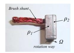
Figure 6. Double layer composition of a brush used in a car starter.
