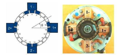
Figure 2. Representation of brushes/commutator contacts for a 4 brushes and 19 segments starter.
