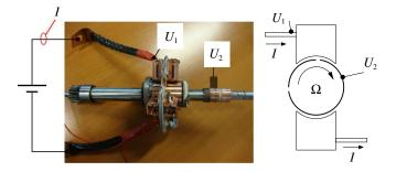
Figure 7. Specific test bench and principle of the Brush-segment sliding contact resistance measurement.
