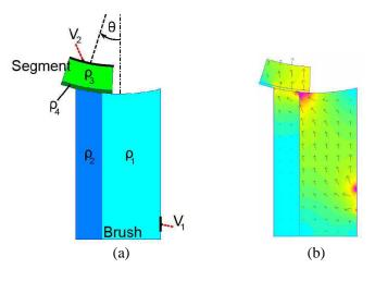
Figure 9. Current flow F.E. model for Brush-segment contact resistance and example of current density for an imposed position  $\theta$ .
