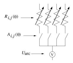
Figure 14. View of the brushes-segment and arc component.
