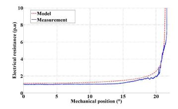
Figure 10. Evolution of a Brush-segment contact resistance with the relative position of the segment calculated by the F.E. model (red) and measured (blue).
