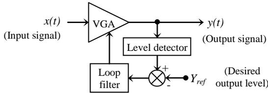
**Fig. 1** Simplified block diagram of a feedback AGC
