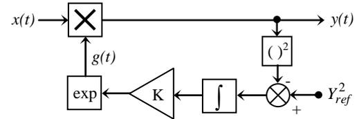
**Fig. 3** Proposed analog feedback AGC
