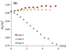
case 2:  $T_0 = 68$  °C,  $d_0 = 99.1 \ \mu\text{m}$ ,  $V_0 = 13 \ \text{m/s}$ ,  $C_0 = 4.5$ ; case 3:  $T_0 = 170$  °C,  $d_0 = 92.1 \ \mu\text{m}$ ,  $V_0 = 13.3 \ \text{m/s}$ ,  $C_0 = 4.8$ )
