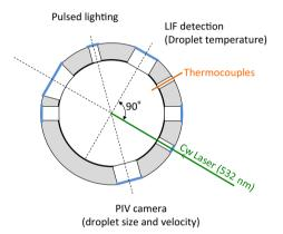
Fig. 2 Optical access for the implementation of the different optical techniques
