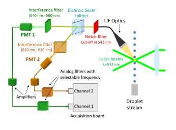
Fig. 4 Schematic view of the 2cLIF system for droplet temperature measurement
