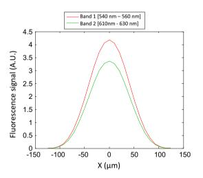
Fig. 15 Evolution of the fluorescence signal as a function of the vertical position of the droplet within the measurement volume (X = 0 corresponds to a droplet centered in the measurement volume)
