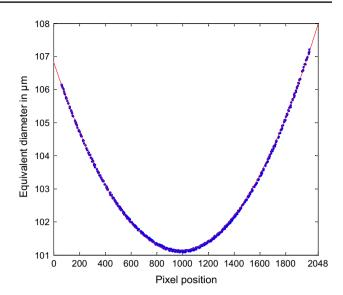
Fig. 18 Droplet size measurements as a function of the vertical position in the images given in pixels. Sizes are obtained without any correction of the image distortion (but using a calibration target to have the magnification factor). In *red*, a second-order polynomial fitted line that can be used to correct the pincushion distortion by assuming that the droplets are in focus in the images during the measurements
