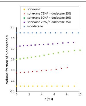
Fig. 27 Evolution of the volume fraction of n-dodecane evaluated from Eq. 10 for the same experimental conditions as in Figs. 25 and 26
