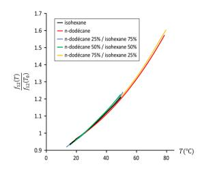
Fig. 6 Calibration curves for n-dodecane/isohexane mixtures
