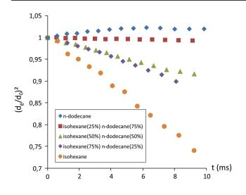
Fig. 25 Evaporation of binary component droplets for similar experimental conditions. Evolution of the droplet size ( $T_0 = 35$  °C,  $d_0 = 115 \ \mu\text{m}, V_0 = 8.5 \ \text{m/s}, C_0 = 6$ )
