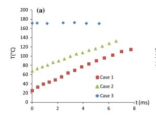
Fig. 22 Evaporation of *n*-dodecane droplets for different injection temperatures. Evolution of the temperature (a), the size (b) (case 1:  $T_0 = 26$  °C,  $d_0 = 97.4$  µm,  $V_0 = 11.8$  m/s,  $C_0 = 4.2$ ;
