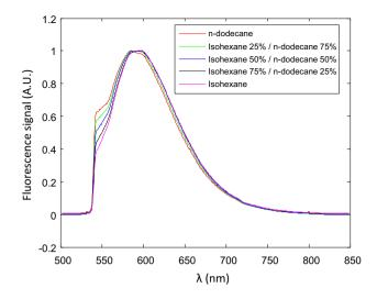
Fig. 8 Emission spectra of pyrromethene 597-C8 at T = 25 °C in several isohexane/*n*-dodecane mixtures
