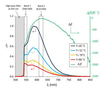
**Fig. 3** Emission spectra of pyrromethene 597-C8 recorded at different temperatures. In *green*, the temperature sensitivity  $\Delta\beta = -T^2 \frac{\partial}{\partial T} \ln (I_f(\lambda)/I_f(\lambda_0))$  with  $\lambda_0 = 630$  nm
