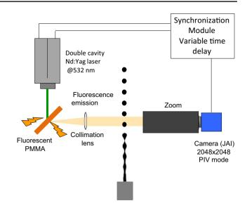
Fig. 16 Experimental setup for the measurement of the droplet diameter by shadowgraphy
