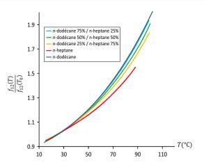
Fig. 7 Calibration curves for *n*-dodecane/*n*-heptane mixtures
