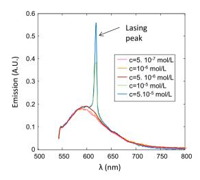
Fig. 10 Emission spectra recorded on 100-µm decane droplets with several concentrations in pyrromethene 597-C8
