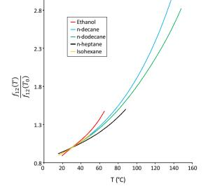
Fig. 5 Calibration curves showing the effect of temperature on the signal ratio  $R_{12}$  ( $T_0$  = 25 °C)
