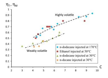
Fig. 24 Influence of the inter-droplet spacing and the fuel volatility on the reduction of the heat and mass transfers
