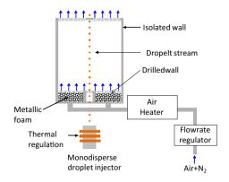
Fig. 1 Schema of the experimental setup: heated enclosure and droplet monodisperse stream
