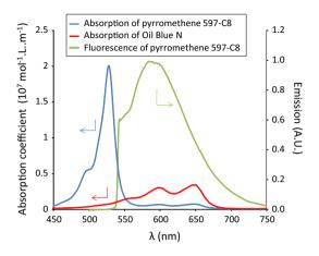
Fig. 11 Absorption and emission spectra of pyrromethene 597-C8 and Oil Blue N
