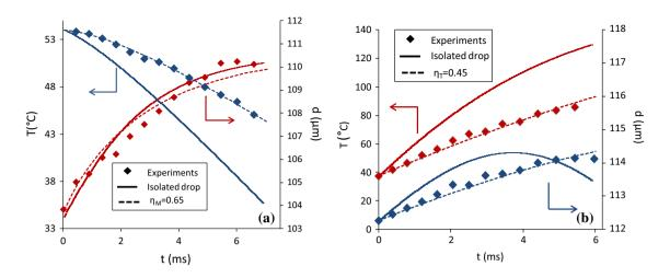
Fig. 23 Evolutions of temperature and size in the case of two droplet streams. a Ethanol ( $T_0 = 35.1$  °C,  $d_0 = 111.6$  µm,  $V_0 = 11.8$  m/s,  $C_0 = 5.4$ ). b *n*-Dodecane ( $T_0 = 37.6$  °C,  $d_0 = 112.3$  µm,  $V_0 = 13.1$  m/s,  $C_0 = 5.9$ )
