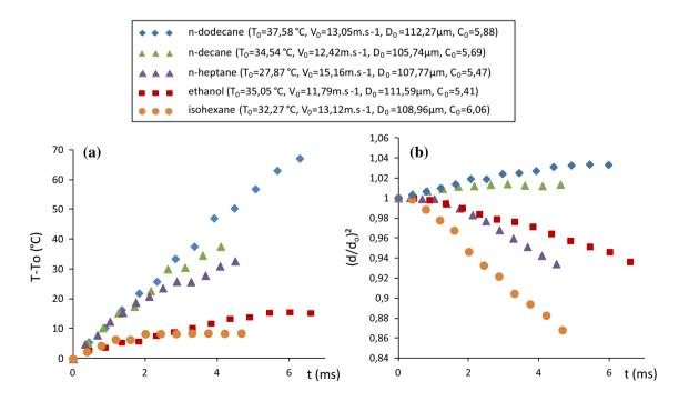
Fig. 21 Evaporation and heating of droplets made of different liquids
