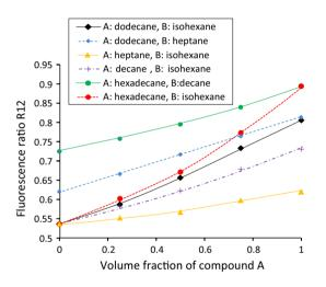
Fig. 9 Evolution of the fluorescence ratio  $R_{12}$  as a function of the volume fraction of several liquid fuels mixed at 25 °C. Spectral bands of detection are those displayed in Fig. 3
