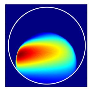
Fig. 14 Fluorescence field viewed by the detection system. Case of a 112- $\mu$ m droplet shifted vertically by 40  $\mu$ m with respect to the measurement volume
