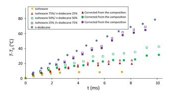
Fig. 26 Evaporation of binary droplets in the same experimental conditions as in Fig. 25. Hollow markers correspond to corrected values of the measurements
