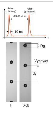
Fig. 17 Principle of the measurement of the droplet diameter and velocity
