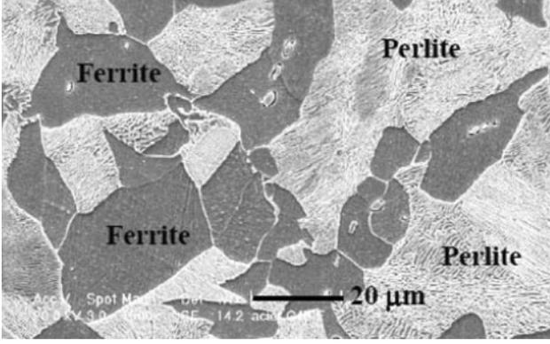
**Fig. 3** Microstructure of the ferrite- perlite steel AISI 1045 [23]
