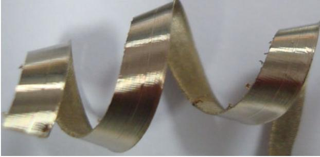
**Fig. 5** Experimental chip morphology: continuous chip without segmentation
