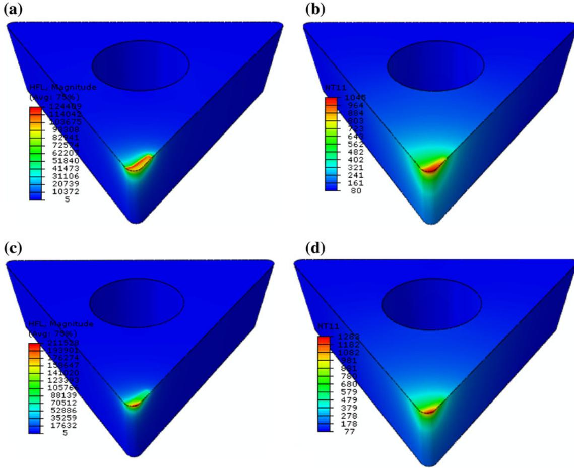
**Fig. 16** Heat flux and temperature distributions in the insert at cutting time equal 5 s: **a** heat flux and **b** temperature fields for applied uniform heat flux, **c** heat flux and **d** temperature fields for applied non-uniform heat flux
