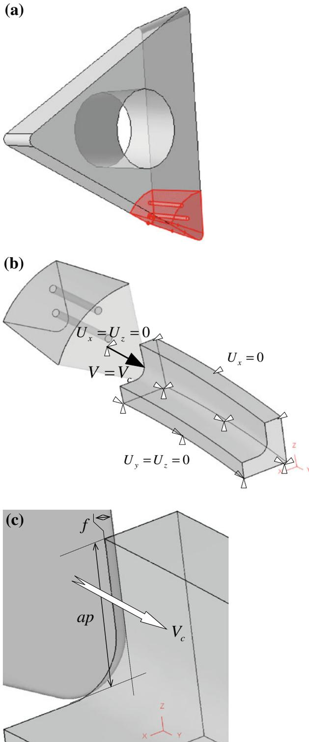
**Fig. 7** First-step FE model for the simulation of the chip formation process [37]: **a** highlighting of the considered part of the cutting tool, **b** initial tool-workpiece configuration with boundary conditions and **c** highlighting of the cutting zone
