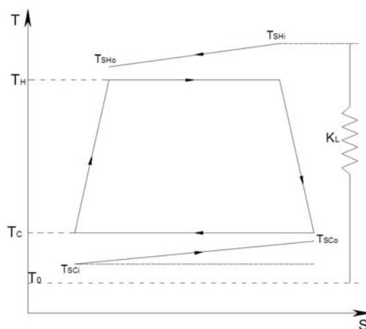
This kind of application is common in industry and of major concern now regarding microcogeneration. Here we assume that the machine is functioning according to the direct cycle represented on Figure 2. This corresponds to a Carnot CHP system, but differs from the one presented recently [28] because we take account here of the finite size of the source and sink, through  $C_H, C_C$ , respectively.
