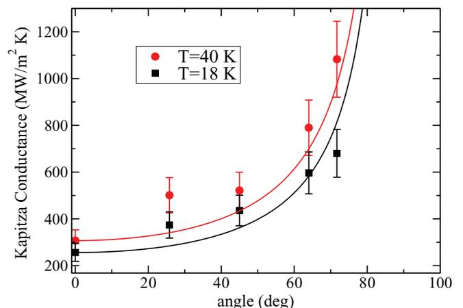
FIG. 8. (Color online) Same as Fig. 7, but for a constant value of the true surface area. The interfacial heights are, respectively,  $h = 21, 34, 43$ , and 45 monolayers for the asperities angles  $\alpha = 25.8, 45, 64$ , and 71.7 deg. The solid lines show the interfacial conductance rescaled by the true surface area:  $G_K = G_K(\alpha = 0)/\cos \alpha$ .
