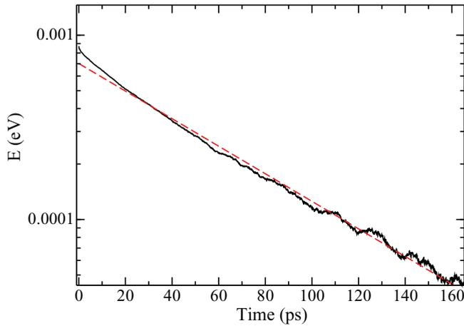
FIG. 2. (Color online) Energy decay of the heated solid obtained using thermal-relaxation simulations. Dashed lines show the exponential fit. The parameters are total length =  $40 a_0$ , temperature  $T = 40$  K, and mass ratio  $m_r = 2$ .
