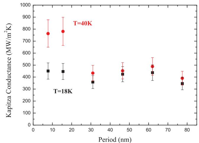
FIG. 3. (Color online) Thermal boundary conductance of isosceles-triangular-shaped interfaces having a roughness height  $h = 32$  MLs, as a function of the period  $p$  defined in Fig. 1. Top:  $T = 40$  K; bottom:  $T = 18$  K. The mass ratio is  $m_r = 2$ .
