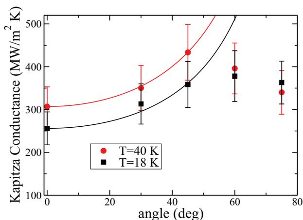
FIG. 7. (Color online) Thermal boundary conductance as a function of the angle of the asperities  $\alpha$ . The height of the asperities is fixed here and equal to 24 ML. The points corresponding to  $\alpha = 0$  denote the conductance of a planar interface. The solid lines show the interfacial conductance rescaled by the true surface area:  $G_K = G_K(\alpha = 0)/\cos \alpha$ . The other parameters are total length = 40  $a_0$  and mass ratio  $m_r = 2$ .
