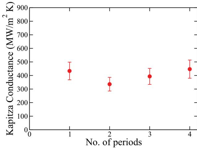
FIG. 4. (Color online) Thermal boundary conductance of isosceles-triangular-shaped interfaces having a roughness height  $h = 32$  MLs and a period  $40 a_0$ , as a function of the No. periods of the superlattice. The temperature is  $T = 40$  K and the mass ratio is  $m_r = 2$ .
