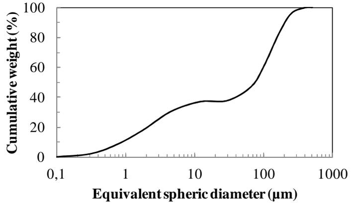
Figure 1 : Particle size distribution of kaolinite - sand mixture.
