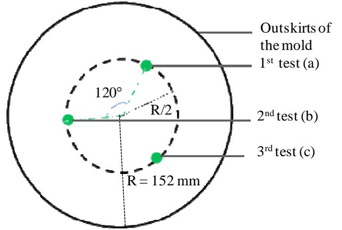
Figure 4: Position of penetration tests in the mold.
