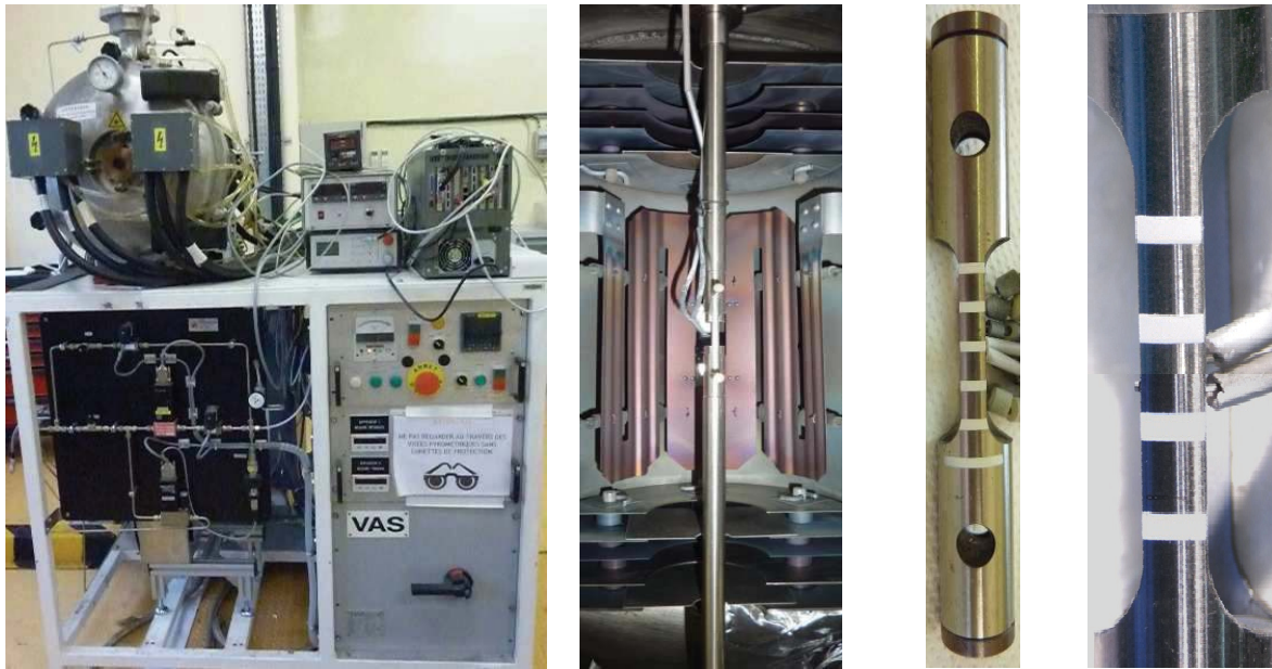
Figure 3: a) ELFE facility b) Inside the furnace and c) Detail of the sample
