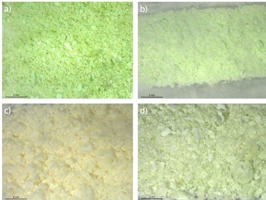
2 Fig. 3. Optical micrographs: (a) ESM, (b) ESMc, (c) ESMa and (d) ESME. ESM, ESMc and ESME share a 3 green appearance, while ESMa appears canary. ESMc and ESMa present a finer appearance than ESM. 4 LEICA microscope (M80, obj x1). Scale bar corresponds to 2 mm.
