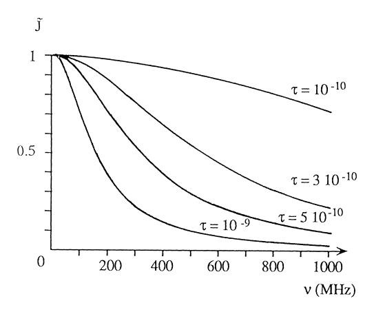
Figure 4. Normalized spectral densities as a function of  $v = \omega/2\pi$  for different values of the correlation time  $\tau$  (in s). They all start from 1 just to highlight their dependence with respect to the measurement frequency.
