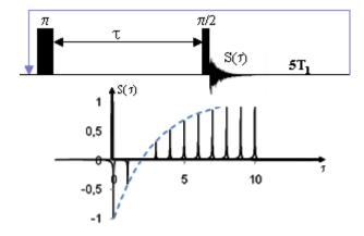
Figure 6. The inversion-recovery experiment. The dynamic range is twice the equilibrium magnetization
