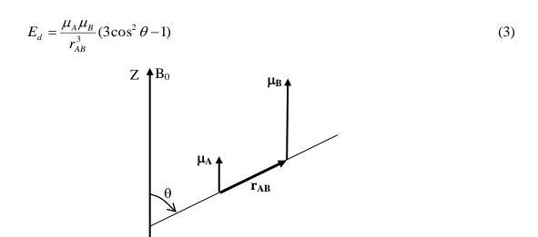
Figure 1. Magnetic dipoles associated with nuclear spins in the presence of B<sub>0</sub>.
