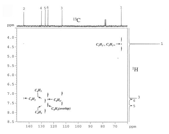
Figure 16. The J-separated HOESY spectrum of the molecule shown in figure 15. Direct (one-bond) correlations are located at the position of <sup>13</sup>C satellites in the proton spectrum. Arrows indicate remote correlations.
