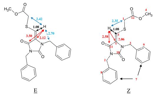
Figure 11. Two isomers with distances (in Å) obtained by quantum chemistry calculations. Solid lines: proton-carbon distances. Dashed lines: proton-proton distances.
