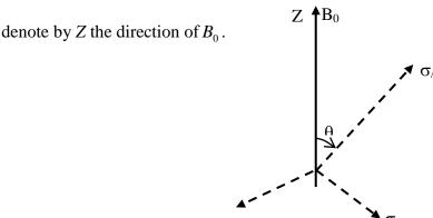
Figure 2. Principal axis system of a shielding tensor assumed to be of axial symmetry.
