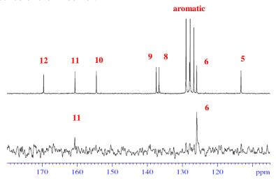
Figure 12. The <sup>13</sup>C responses (bottom) obtained by selectively inverting H<sub>5</sub> (bound to a carbon-12); they lead to the cross-relaxation rates  $\sigma_{H_5-C_6}$  and  $\sigma_{H_5-C_{11}}$ . A reference carbon-13 spectrum is shown at the top.
