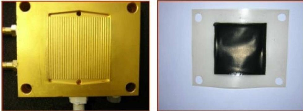
Flow field plates (gold plated brass; the anode and the cathode plates are symmetrical with 28 parallel channels) and MEA (Johnson Matthey Technologies; Ageom = 23.88 cm<sup>2</sup>) of the single cell used for experimental studies.
