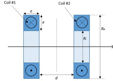
Fig. 2. Schematic representation of the Helmholtz coil system.
