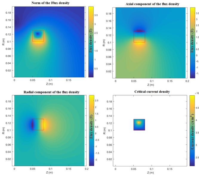
Fig. 3. Plot of the magnetic flux density and the critical current density maps obtained via Matlab simulations. This plot correspond to the optimal designed system ( $d=0.1$  m and  $e=0.031$  m)
