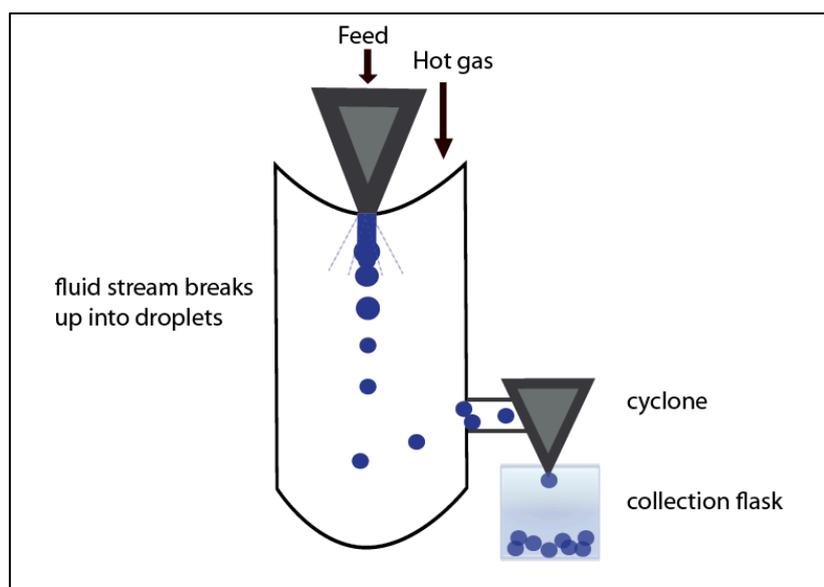
**Figure 2.** Basic schema of a concurrent spray dryer.
