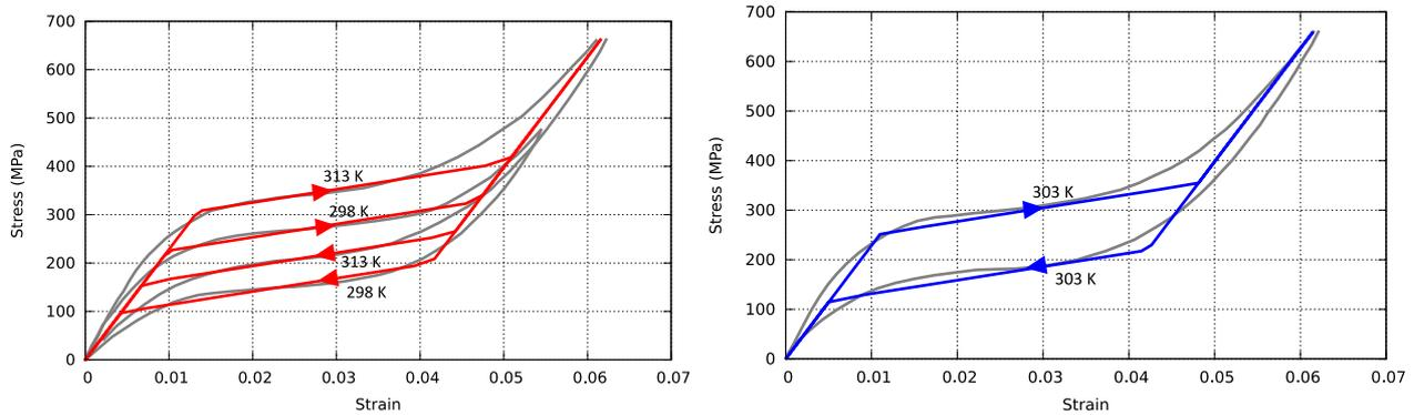
Figure 2. Comparison between simulation using the identified model parameters and the experimental response in uniaxial tension. Identification at 298 K and 313 K (a) and validation at 303 K (b).
