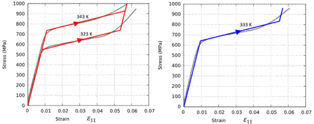
Figure 1. Comparison between the simulated response and the experimental data a) for isothermal tests at the two temperatures utilized in the parameter identification procedure (323 K and 343 K). b) Experimental validation for an isothermal test at 333 K.
