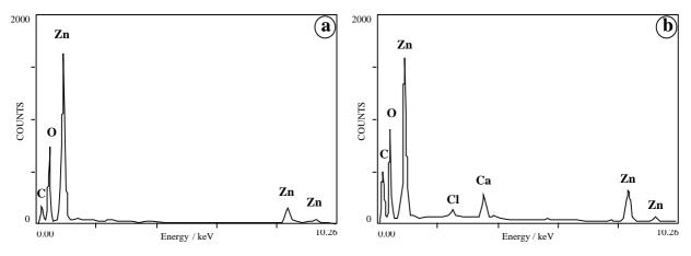
Fig. 2: SEM-EDS spectra of the zinc carbonate hydroxide samples
