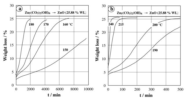
Fig. 6 : Isothermal treatment of RFS between 150 and 240  $^{\circ}$ C.
