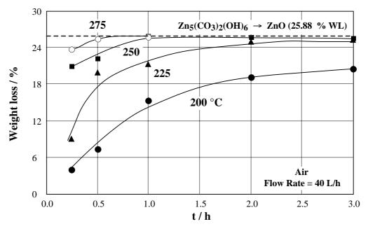
Fig. 9: Treatment of RFS between 200 and 275 °C at different times.
