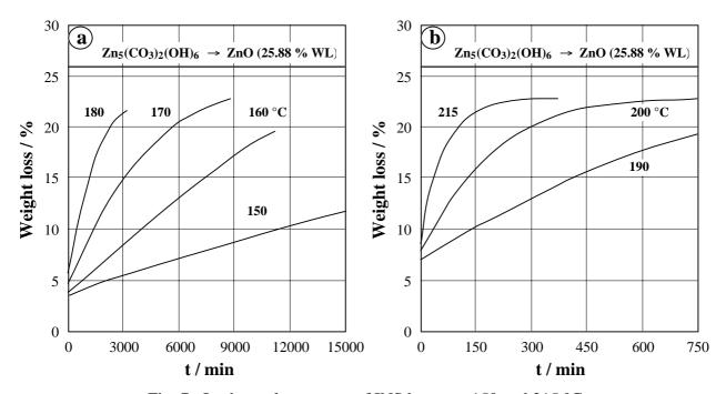
Fig. 7: Isothermal treatment of INS between 150 and 215 °C.
