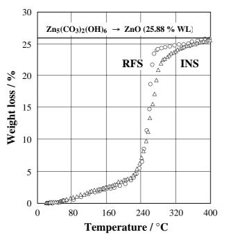
Fig. 4: TG non isothermal treatment of samples.
