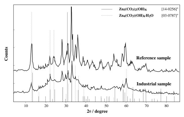
Fig. 1: XRD results of zinc carbonate hydroxide samples.
