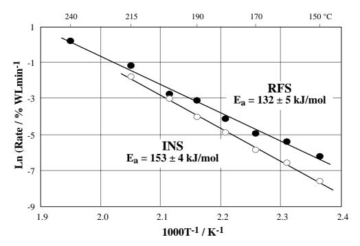
Fig. 8: Arrhenius diagrams of decomposition of both samples.
