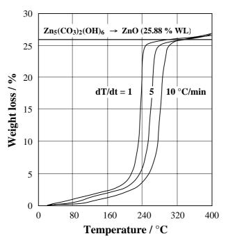
Fig. 5 : Treatment of RFS at different heating rates.
