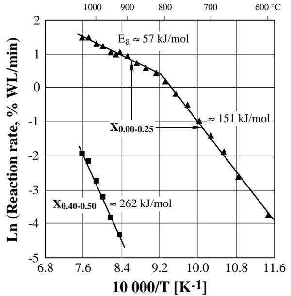
Figure 8 : Example of Arrhenius plot of the chromite oxychlorination.
