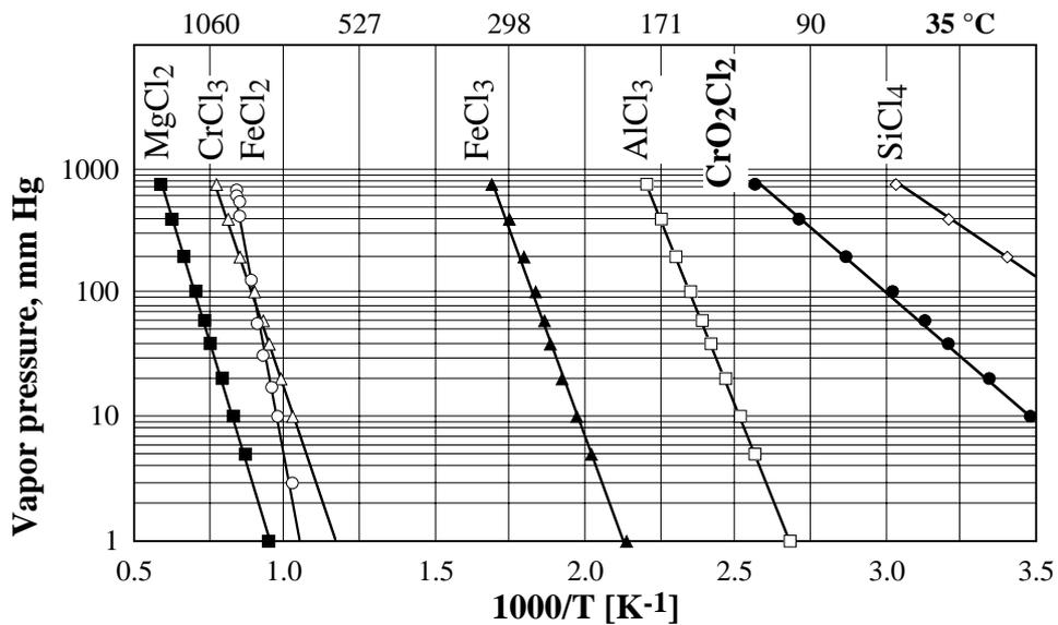
Figure 2 : Evolution of vapor pressure of several chlorides as a function of temperature<sup>[8,9]</sup>.
