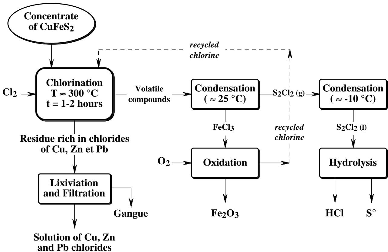
Fig. 22 : Suggested flow-sheet for the extraction of valuable metal chlorides by chlorination.
