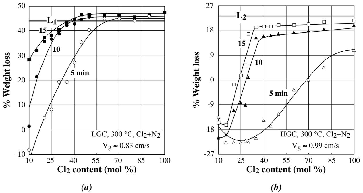
Fig. 11 : Effects of the chlorine content in the gas mixture and reaction time on the chlorination of (a) LGC and (b) HGC.
