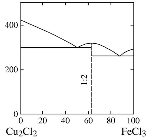
Fig. 18 : Phases' diagram of CuCl-FeCl<sub>3</sub> system.[17]
