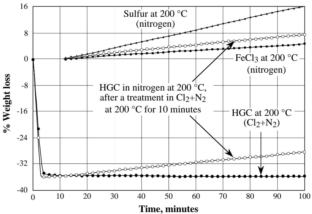
Fig. 19 : Behavior of chlorination residue of HGC, of sulfur and FeCl<sub>3</sub> at 200 °C in N<sub>2</sub>.
