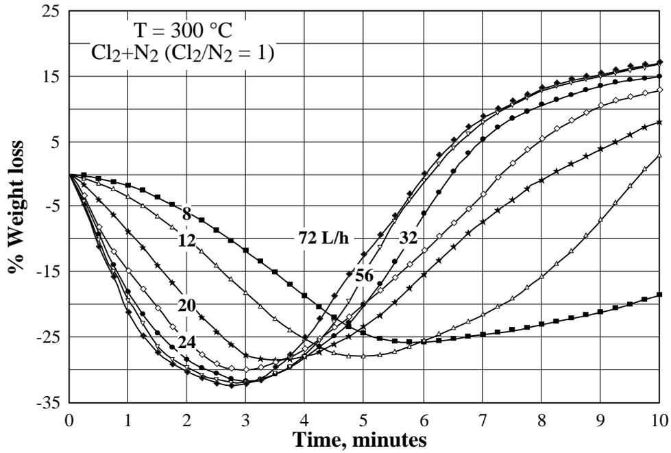
Fig. 7 : Isotherms of chlorination of HGC with Cl<sub>2</sub>+N<sub>2</sub> using various gas flow rates.
