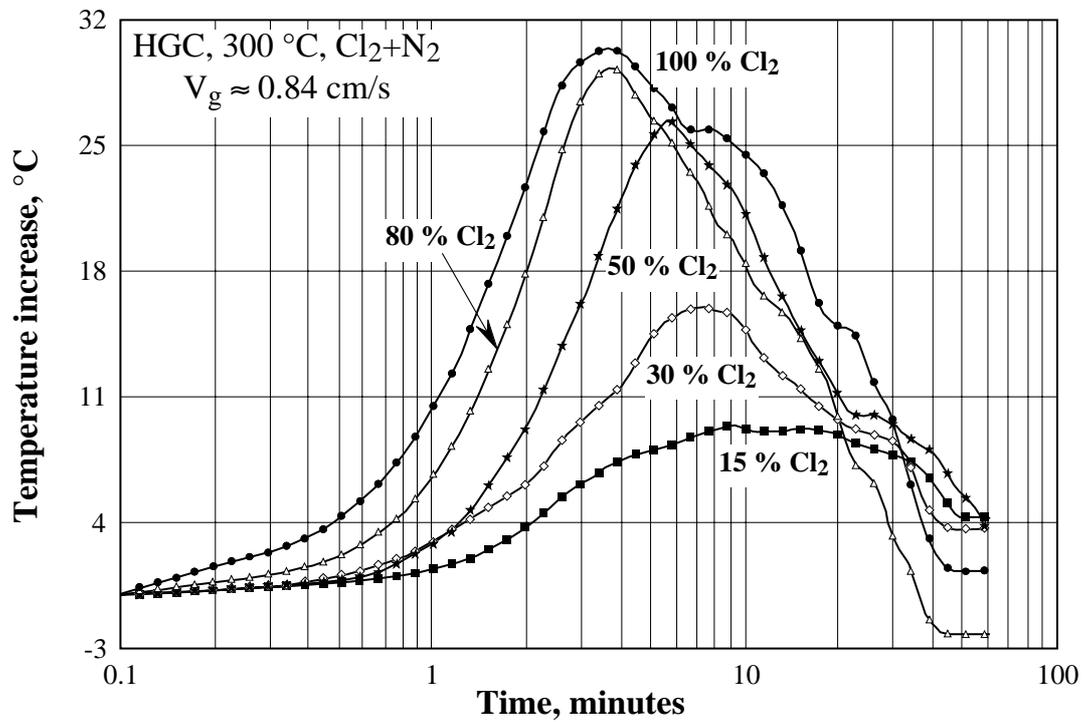
Fig. 21 : Increase of temperature during the chlorination of HGC in a horizontal experimental set using different chlorine contents in Cl<sub>2</sub>+N<sub>2</sub> gas mixture.
