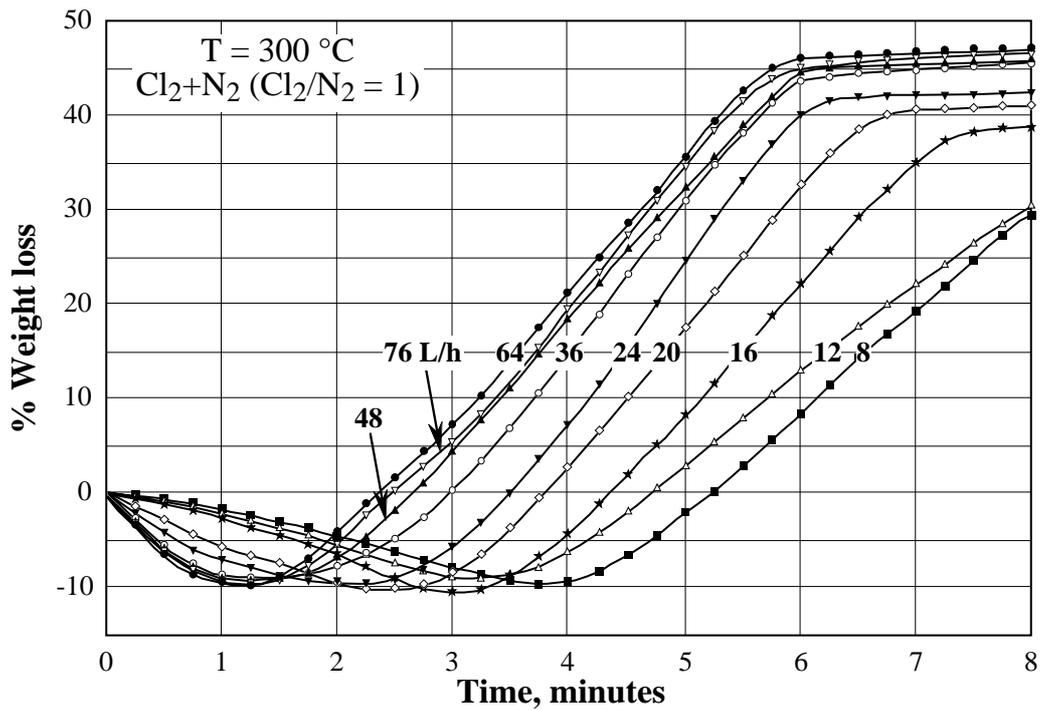
Fig. 6 : Isotherms of chlorination of LGC with  $\text{Cl}_2 + \text{N}_2$  using various gas flow rates.
