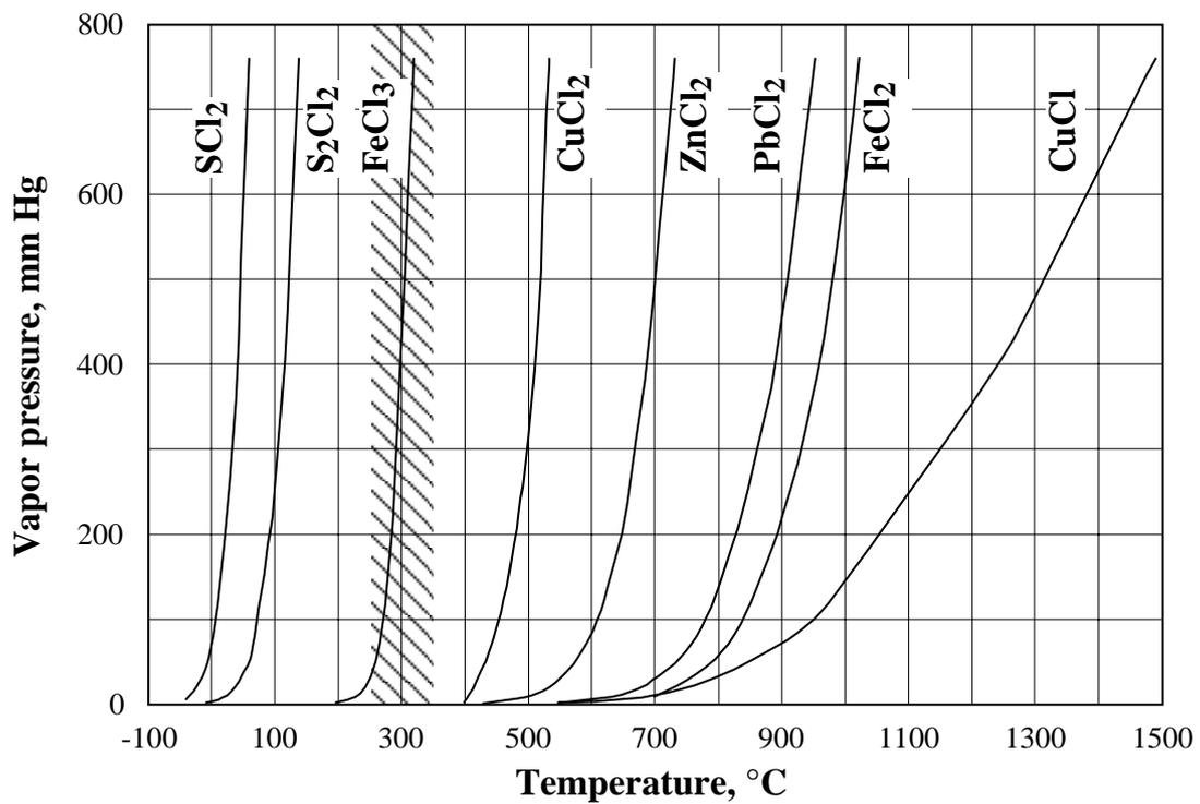
Fig. 4 : Evolution of vapor pressure of several chlorides<sup>[16]</sup>.
