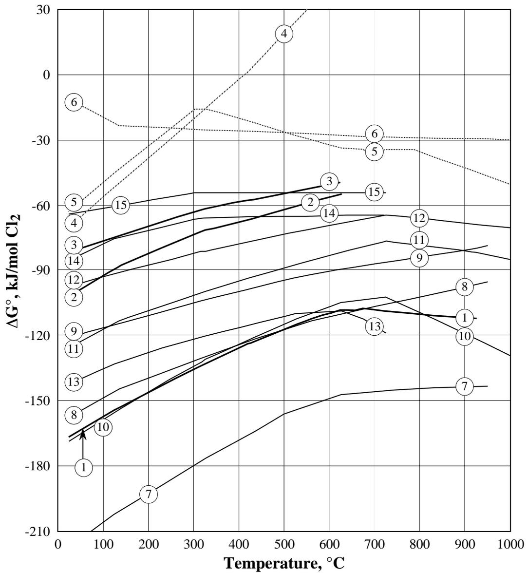
Fig. 3 : Evolution of the standard free energy changes ( $\Delta G^\circ$ ) as a function of temperature for the chlorination of the compounds contained in the chalcopyrite concentrates<sup>[14,15]</sup>.
