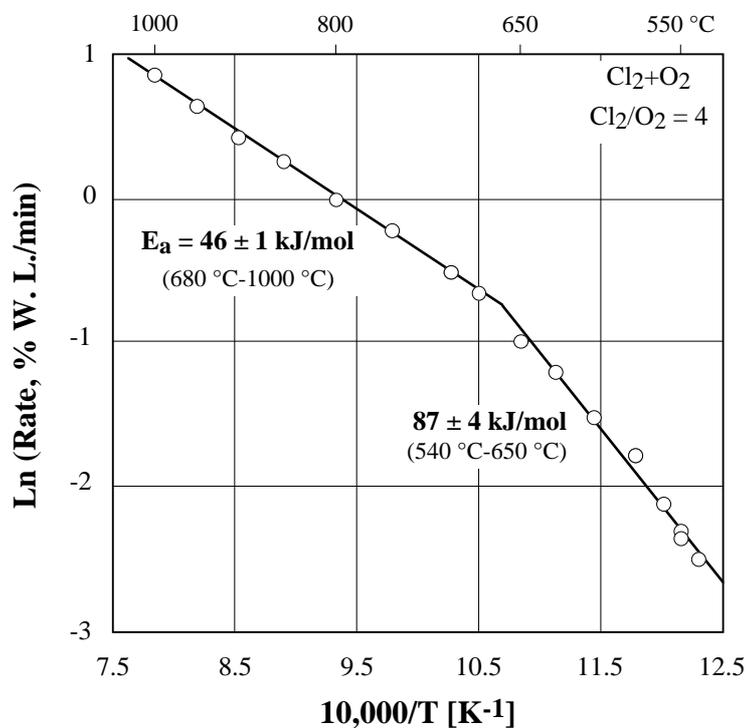
Fig. 15- Arrhenius plot of chlorination of  $\text{Cr}_2\text{O}_3$  by  $\text{Cl}_2+\text{O}_2$ .
