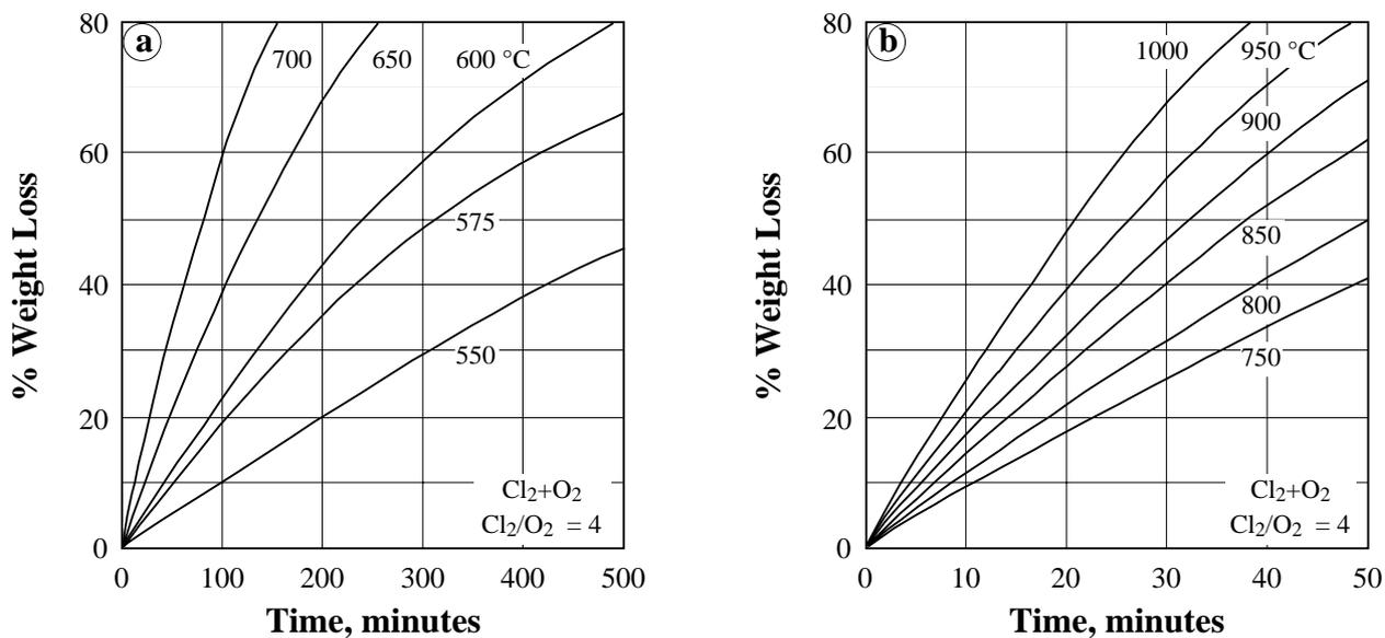
Fig. 14- Isotherms of chlorination of  $\text{Cr}_2\text{O}_3$  with  $\text{Cl}_2+\text{O}_2$  for (a)  $T \leq 700^\circ\text{C}$  and (b)  $T \geq 750^\circ\text{C}$ .
