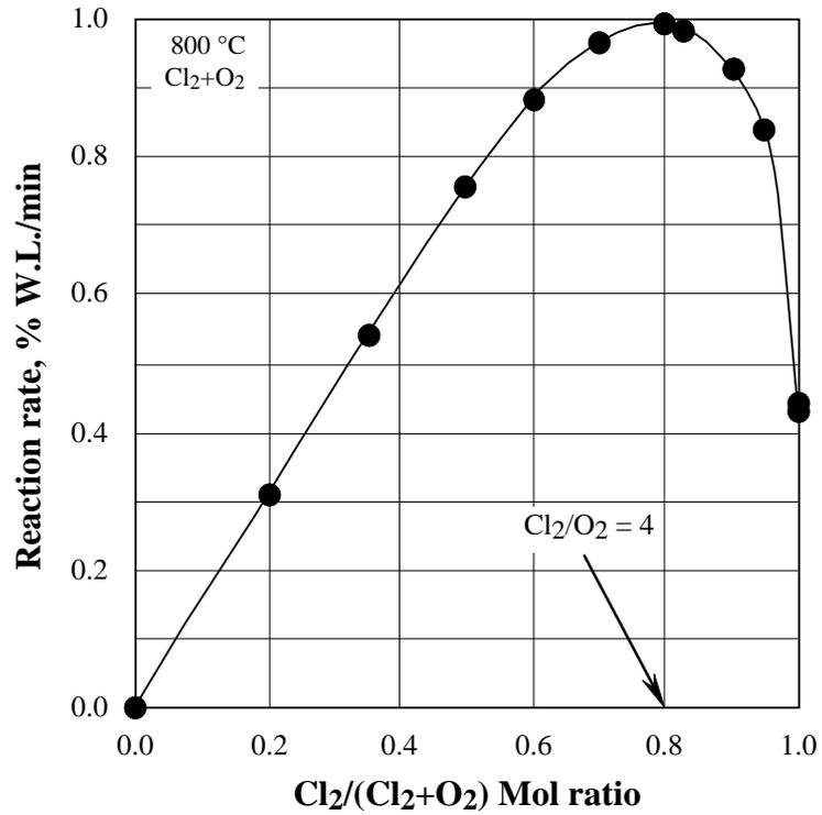
Fig. 10- Effect of Cl<sub>2</sub>/(Cl<sub>2</sub>+O<sub>2</sub>) molar ratio on the reaction rate of Cr<sub>2</sub>O<sub>3</sub> oxychlorination.
