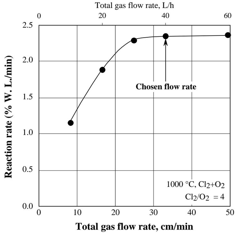
Fig. 9- Chlorination rate of Cr<sub>2</sub>O<sub>3</sub> as a function of flow rate of the Cl<sub>2</sub>+O<sub>2</sub> mixture.
