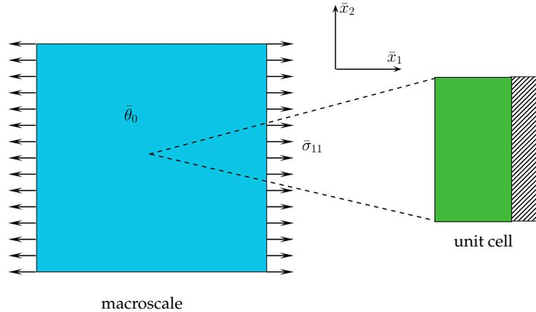
Figure 3: Multilayered composite: Uniaxial response under isothermal conditions.
