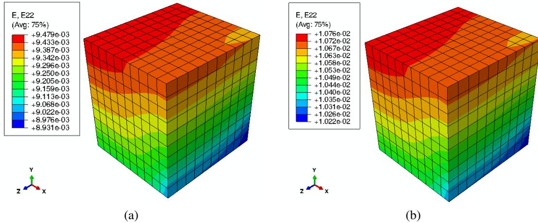
Figure 9: Strain  $\bar{\epsilon}_{22}$  distribution in the macrostructure for total analysis time of a) 200 s and b) 20000 s. Composite with 20% epoxy volume fraction.
