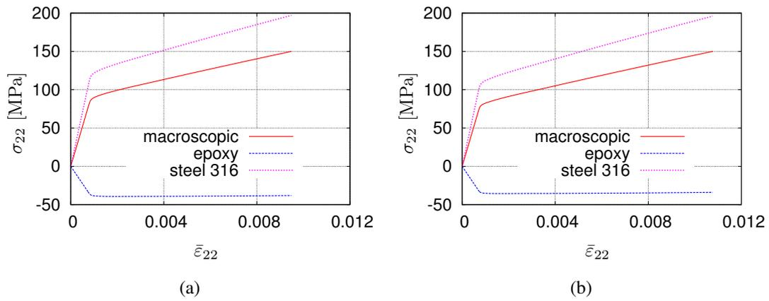
Figure 11: Evolution of macroscopic and microscopic stresses with strain at the centroid of the element A (Figure 7<sub>a</sub>) for total analysis time of a) 200 s and b) 20000 s. Composite with 20% epoxy volume fraction.
