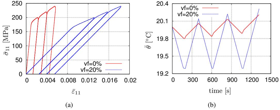
Figure 6: Uniaxial loading (1 MPa/s) of multilayered composite under adiabatic conditions: (a) macroscopic stress-strain curve and (b) evolution of temperature with time for two epoxy volume fractions.
