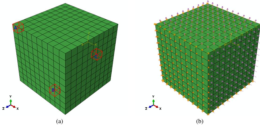
Figure 7: (a) Finite element meshing of macrostructure. (b) Boundary and loading conditions on the meshed macrostructure.
