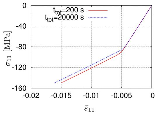
Figure 12: Macroscopic stress-strain in the direction 1 at the centroid of the element B (Figure 7<sub>a</sub>) for two different loading durations. Composite with 20% epoxy volume fraction.
