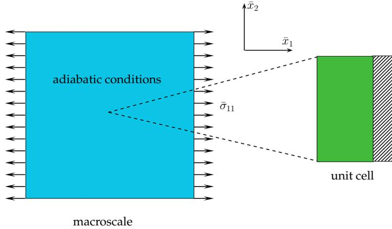
Figure 5: Multilayered composite: Uniaxial response under adiabatic conditions.
