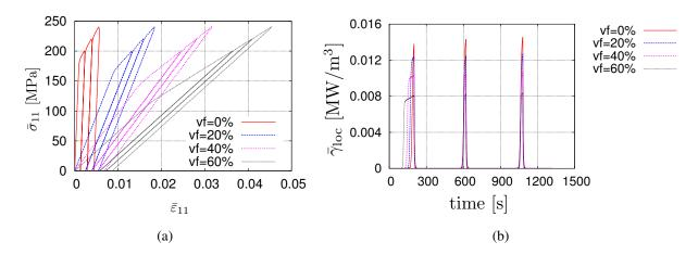
Figure 4: Uniaxial loading (1 MPa/s) of multilayered composite under isothermal conditions: (a) macroscopic stress-strain curve and (b) evolution of macroscopic local dissipation with time for four epoxy volume fractions.
