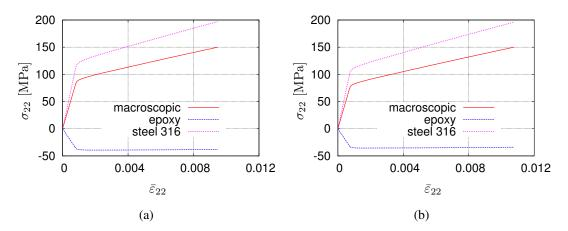
Figure 11: Evolution of macroscopic and microscopic stresses with strain at the centroid of the element A (Figure  $7_a$ ) for total analysis time of a) 200 s and b) 20000 s. Composite with 20% epoxy volume fraction.
