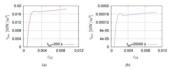
Figure 13: Macroscopic local dissipation distribution at the centroid of the element C (Figure  $7_a$ ) for total analysis time of a) 200 s and b) 20000 s. Composite with 20% epoxy volume fraction.
