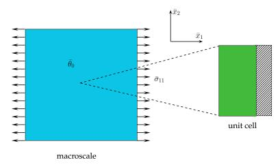
Figure 3: Multilayered composite: Uniaxial response under isothermal conditions.
