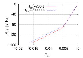
Figure 12: Macroscopic stress-strain in the direction 1 at the centroid of the element B (Figure  $7_a$ ) for two different loading durations. Composite with 20% epoxy volume fraction.
