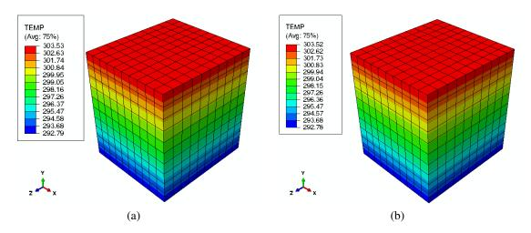
Figure 10: Temperature distribution (in K) in the macrostructure for total analysis time of a) 200 s and b) 20000 s. Composite with 20% epoxy volume fraction.
