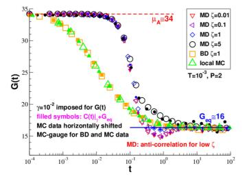
FIG. 4. (Color online) Stress relaxation modulus G(t) (open symbols) and rescaled autocorrelation function  $C(t)|_{\gamma} + G_{eq}$  (filled symbols) for MD simulations for several friction constants  $\zeta$ , BD simulations with  $\zeta = 1$ , and local MC moves. Shifting horizontally the MC data by a factor of 1/8000 allows us to bring them to a collapse onto the BD data.
