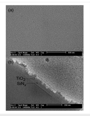
Figure 1: SEM images of the (a) top surface and (b) cross section of the sol–gel TiO<sub>2</sub> films grown on 75 nm thick SiN<sub>x</sub>/SLG after annealing at 450 °C.
