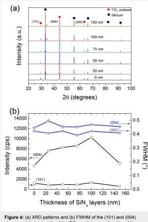
planes and their intensity of the TiO<sub>2</sub> coatings as a function of the thickness of the SiN<sub>x</sub>/SLG films.
