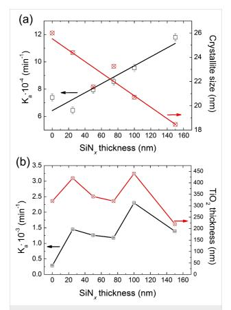
**Figure 5:** Evolution of the kinetics of the degradation rate of OII. The crystallite size and TiO<sub>2</sub> thickness of (a) a SG-TiO<sub>2</sub> film and (b) the magnetron sputtered TiO<sub>2</sub> film as a function of SiN<sub>x</sub> thickness.
