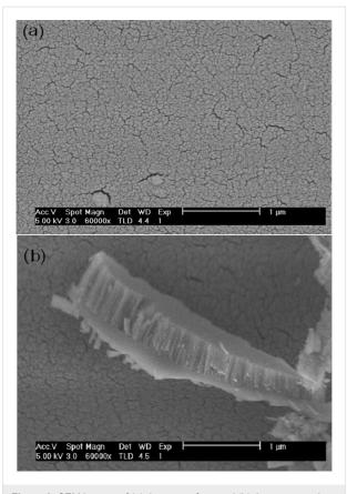
Figure 2: SEM images of (a) the top surface and (b) the cross-section of the magnetron sputtered  $TiO_2$  films grown on SiN<sub>x</sub>/SLG after annealing at 450 °C.
