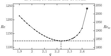
FIGURE 5. For  $n_C = 0.5$ ,  $\lambda = 1$ . Onset curves of the saddle-node bifurcations Reynolds numbers  $Re(q; n_C, \lambda)$  (left ordinate axis) and  $Re_w(q; n_C, \lambda)$  (right ordinate axis); dashed lines, critical wavenumber and Reynolds numbers;  $\star$ , solution found by RPN2010.
