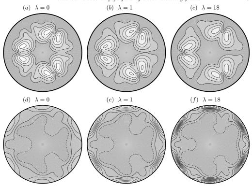
FIGURE 12. For  $n_C=0.5$ , for various values of  $\lambda$  as indicated. (a,b,c): rms axial velocity  $w'(r,\theta)$ ; continuous lines, 5 regularly spaced contours  $w'=0.025\overline{W}$  to  $0.125\overline{W}$ ; dark gray (resp. light gray), low (resp. high) values. (d,e,f):  $\langle \Gamma_2 \rangle_z$ ; dashed line, first iso contour  $\Gamma_2=0.5$ ; continuous lines, 10 regularly spaced contours  $\Gamma_2=1.5$  (near the center) to 15 (near the pipe wall).
