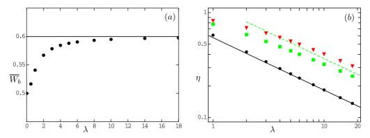
FIGURE 3. (Colour online) For  $n_C = 0.5$ . (a):  $\circ$ , bulk velocity of the base flows; full line, power-law fluid bulk velocity of the base flows. (b):  $\circ$ , wall viscosity of the base flows; full line, power-law fluid wall viscosity of the base flows;  $\Box$ , bulk average mean viscosity of the base flows; dashed line, power-law fluid mean viscosity of the base flows;  $\nabla$ , bulk average mean viscosity of the critical waves discussed in §5.3.
