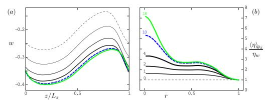
FIGURE 13. (Colour online) For  $n_C=0.5$ , for the critical waves corresponding to the values of  $\lambda$  indicated in figure (b). (a): axial velocity  $w=v_z-W_b$  at  $r=0.59,~\theta=1.29$ . (b): ratio of the viscosity averaged over  $\theta$  and z to the wall viscosity.
