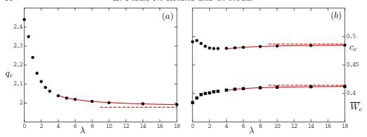
FIGURE 9. (Colour online) For  $n_C=0.5$ . (a):  $\circ$ , critical wavenumber; (b):  $\circ$ , critical phase velocity;  $\square$ , critical bulk velocity. Curves, fits computed for  $\lambda \geqslant 6$ ; dashed lines, asymptotic values.
