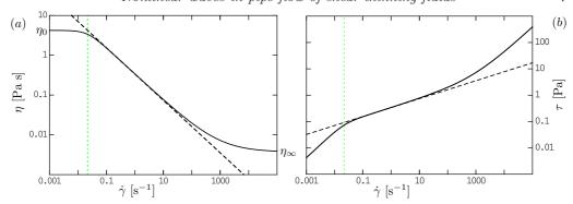
FIGURE 1. (Colour online) Flow curves of the 0.125% PAA fluid studied by Escudier et al. (2009): (a) viscosity (b) shear stress vs shear rate. Continuous curves, Carreau's model (2.6) with  $\eta_0 = 4.22$  Pa s,  $\eta_{\infty} = 0.00372$  Pa s,  $\lambda_C = 45.8$  s,  $n_C = 0.34$ ; dashed lines, power-law model; vertical dotted lines, characteristic shear rate  $\dot{\gamma} = 1/\lambda_C$  for the onset of shear-thinning.
