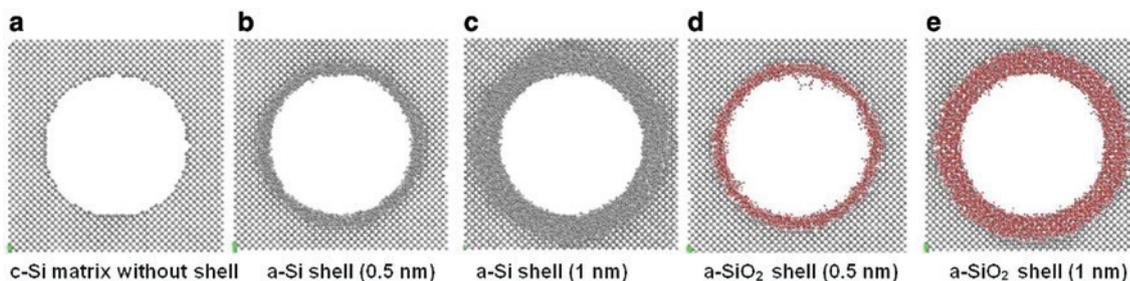
**Figure 1:** Cross sections of Si membranes with cylindrical pores without and with shells: (a) no shell, (b) amorphous Silicon shell with 0.5 nm thickness, (c) amorphous Silicon shell with 1 nm thickness, (d) amorphous SiO<sub>2</sub> shell with 0.5 nm thickness, and (e) amorphous SiO<sub>2</sub> shell with 1 nm thickness. Grey atoms represent silicon and red the oxygen.
