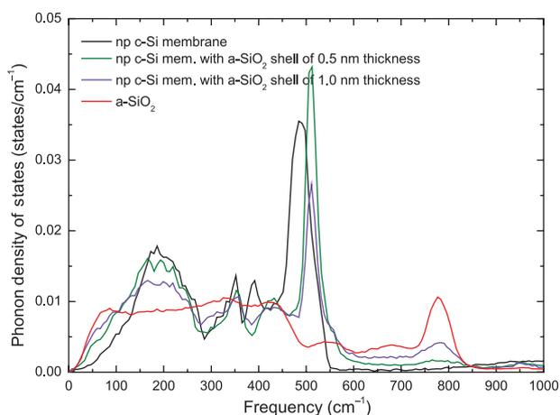
**Figure 4:** Comparison of the phonon density of states of several nanoporous systems with and without a-SiO<sub>2</sub> shells around the pores.
