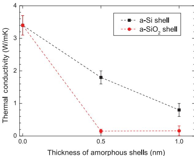
**Figure 2:** Thermal conductivity of nanoporous silicon membranes and the influence of amorphous shell around the pores depending on the amorphous material and the thickness of the shell. The black squares is for a-Si and the red circles for the a-SiO<sub>2</sub> around the pores. Two shell thickness are studied: 0.5 and 1.0 nm.
