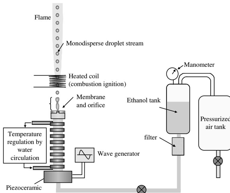
Fig. 1. Experimental arrangement.
