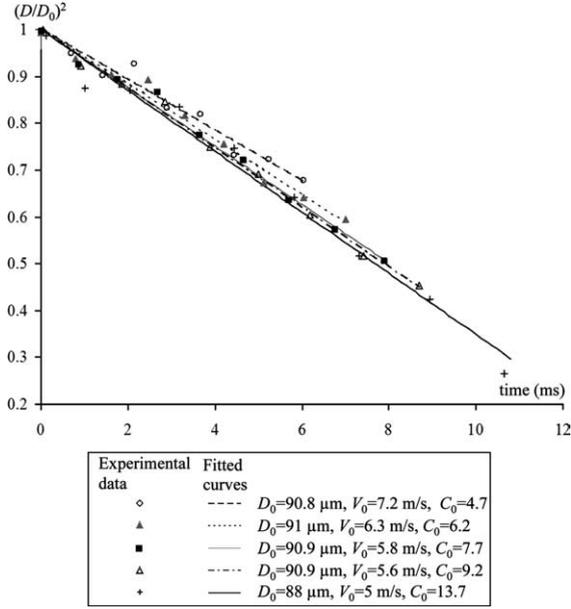
Fig. 8. Temporal evolution of the squared diameter for different distance parameters obtained by successive electrostatic deviation of a monodisperse droplet stream ( $D = 91 \mu\text{m}$ ,  $V = 7.5 \text{ m/s}$ ).
