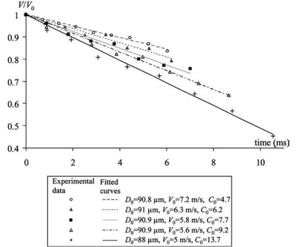
Fig. 7. Temporal evolution of the velocity for different distance parameters obtained by successive electrostatic deviation of a monodisperse droplet stream ( $D = 91 \mu\text{m}$ ,  $V = 7.5 \text{ m/s}$ ).
