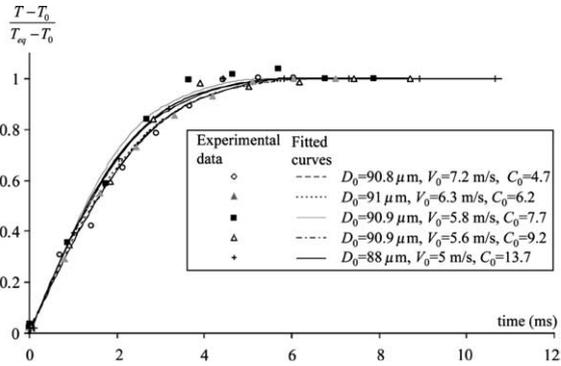
Fig. 9. Temporal evolution of the temperature for different distance parameters obtained by successive electrostatic deviation of a monodisperse droplet stream ( $D = 91 \mu\text{m}$ ,  $V = 7.5 \text{ m/s}$ ).
