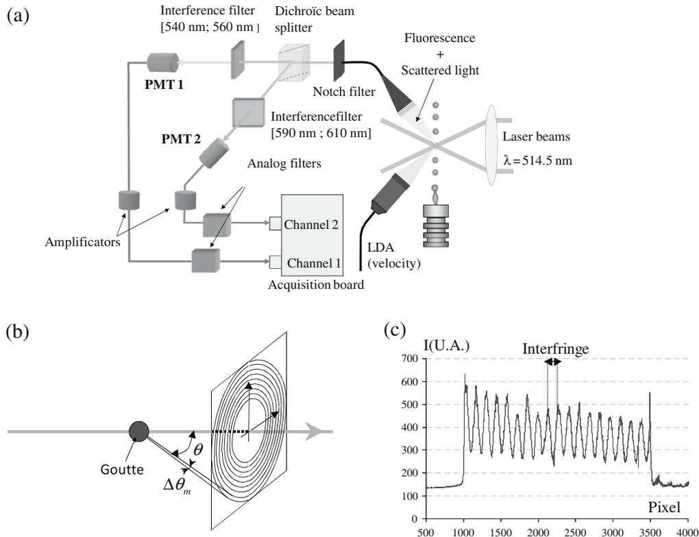
Fig. 2. (a) 2cLIF optical set-up. (b and c) Schematic view of the interference pattern in the forward scattering direction used for droplet size measurement ( $\theta$  scattering angle;  $\Delta\theta_m$  angular interfringe).
