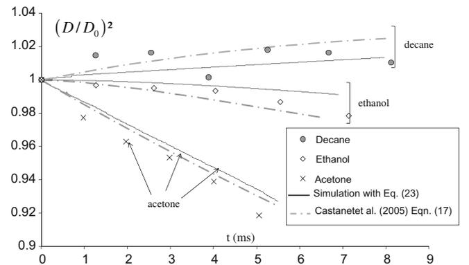
Fig. 8. Temporal evolution of the droplet size in the case of acetone ( $V_0 = 10.6$  m/s,  $D_0 = 122.6$   $\mu\text{m}$ ,  $T_0 = 26$   $^\circ\text{C}$ ), ethanol ( $V_0 = 9$  m/s,  $D_0 = 119.6$   $\mu\text{m}$ ,  $T_0 = 29.7$   $^\circ\text{C}$ ) and dodecane ( $V_0 = 10.8$  m/s,  $D_0 = 121.5$   $\mu\text{m}$ ,  $T_0 = 30$   $^\circ\text{C}$ ) evaporating droplet. Comparison between the experimental results and Eq. (23) and the existing correlations of Castanet et al. [15] (Eq. (17)).
