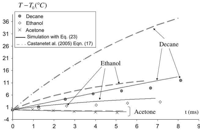
**Fig. 9.** Temporal evolution of the droplet temperature in the case ( $V_0 = 10.6$  m/s,  $D_0 = 122.6$   $\mu\text{m}$ ,  $T_0 = 26$   $^\circ\text{C}$ ), ethanol ( $V_0 = 9$  m/s,  $D_0 = 119.6$   $\mu\text{m}$ ,  $T_0 = 29.7$   $^\circ\text{C}$ ) and dodecane ( $V_0 = 10.8$  m/s,  $D_0 = 121.5$   $\mu\text{m}$ ,  $T_0 = 30$   $^\circ\text{C}$ ) evaporating droplet. Comparison between the experimental results and Eq. (23) and the existing correlations of Castanet et al. [15] (Eq. (17)).
