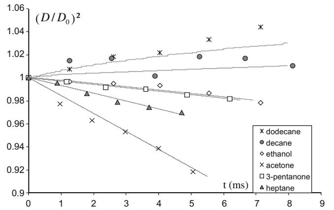
**Fig. 3.** Time evolution of the normalized square diameter for the different droplet streams (dots: experimental data, lines: simulations resulting from the inversion procedure) (initial conditions given in Table 1).
