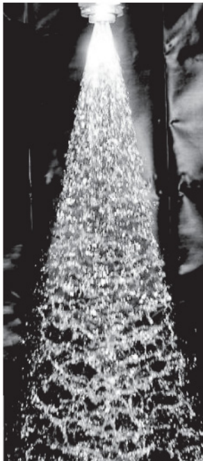
FIG. 1. Sketch of the nozzle orifice and photograph of the experimental setup (Lechler nozzle ref. 665-042, 8 bars). The orifice of the nozzle is made up of two identical circular segments pieced together ( 2a = 977 \mu\text{m} and 2b = 646 \mu\text{m} for ref. 665-042).
