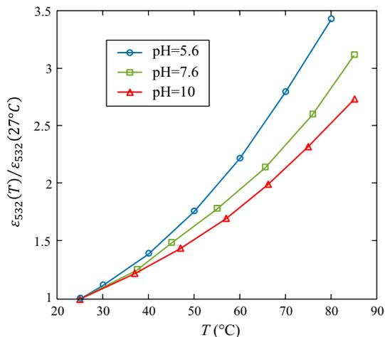
**Fig. 5** Influence of the temperature on the absorption coefficient of FL at 532 nm taking as a reference  $T_0 = 27^\circ\text{C}$
