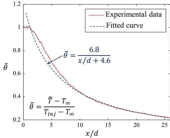
**Fig. 17** Evolution of the normalized mean temperature  $\bar{\theta}$  along the centerline of the turbulent jet.  $\bar{T}$  is the time-averaged temperature,  $x/d$  is the reduced distance to the injector with  $d$  the diameter of the injection nozzle. ( $d = 3$  mm,  $T_{inj} = 63$  °C and  $T_{\infty} = 22$  °C)
