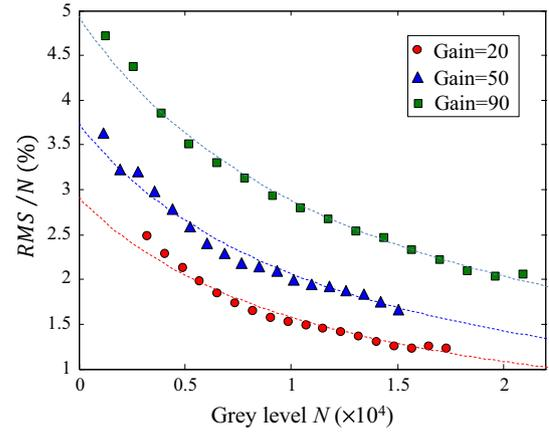
**Fig. 11** Inverse of the signal-to-noise ratio of the camera at several gains of amplification. Dotted lines correspond to the fitting of the experimental data by a function of type  $y(x) = a/(x + b)$ , where  $a$  and  $b$  are two fitted parameters
