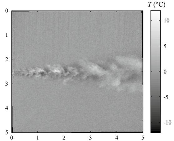
**Fig. 18** Typical instantaneous temperature fluctuations measured in the turbulent heated jet. This image is obtained by subtracting the average temperature derived from two hundreds of images to the instantaneous temperature field in Fig. 15c
