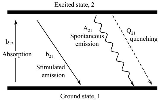
**Fig. 1** A two-level diagram of laser-induced fluorescence
