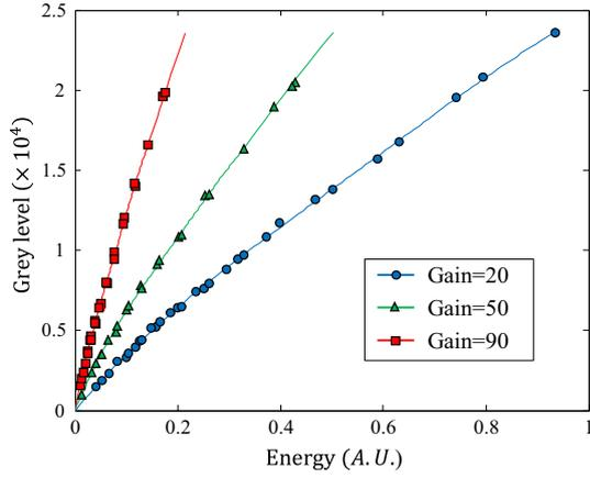
**Fig. 10** Response of ICCD cameras to light irradiance
