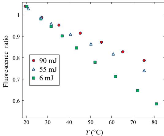
**Fig. 14** Influence of the energy of the laser pulses on the temperature dependence of the fluorescence ratio in the application of the 2c/1d method with KR
