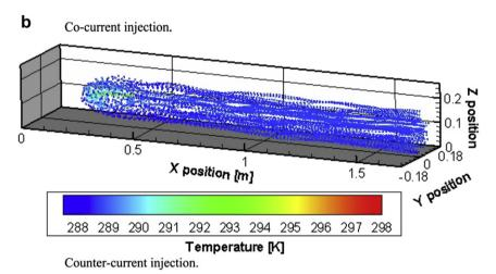
**Fig. 2.** Typical trajectories of 25 μm droplets in an air flow with average velocity of 1 m/s, from a preliminary academical study. Droplets are injected with initial velocity of 10 m/s in a cone with angle 72° in co-current direction (Fig. 2a) and counter-current direction (Fig. 2b).
