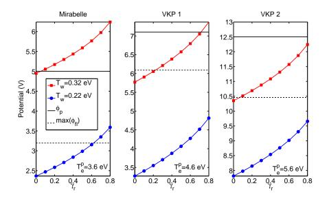
FIG. 4. Average floating potential obtained with Eq. 17 assuming  $T_w = T_e^e$  and using data from Tab. I. Left: Mirabelle experiment, center: VKP 1, right: VKP 2. The floating potential  $\varphi_{fl,max}$  corresponds to the maximum of the probe floating potential obtained experimentally. The plasma potential  $\varphi_p$  was obtained from cold probe analysis.
