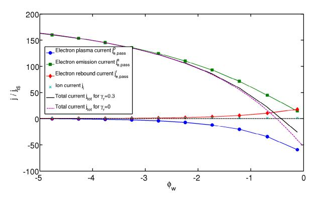
FIG. 3. Example of the different passing current densities flowing through an emissive surface under space-charge regime. The current densities are normalized to the ion saturation current density. The calculation was performed for an Argon plasma with  $n_0 = 1 \times 10^{18} \text{ m}^{-3} T_e^p = 5 \text{ eV}$ ,  $T_e^e = T_w = 0.31 \text{ eV}$ ,  $\gamma_r = 0.3$ ,  $\varphi_{\text{work}} = 4.5 \text{ eV}$  and  $A_0 = 1.2 \times 10^6 \text{ Am}^{-2} \text{K}^{-2}$  (tungsten surface).
