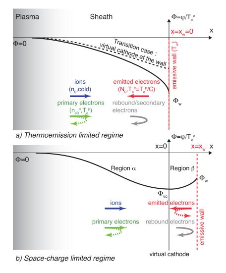
FIG. 1. Schematic of 1-D static sheath under (a) thermoemission limited regime (b) space-charge limited regime. See text for details.
