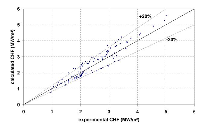
Figure 10a : Comparison between data and calculated CHF using (22), upstream
