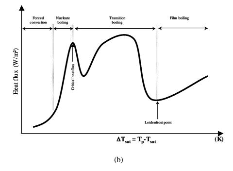
Figure 1 : Shape of the boiling curve in impinging jet experiments (a) parallel flow zone of the jet (b) impinging zone of the jet
