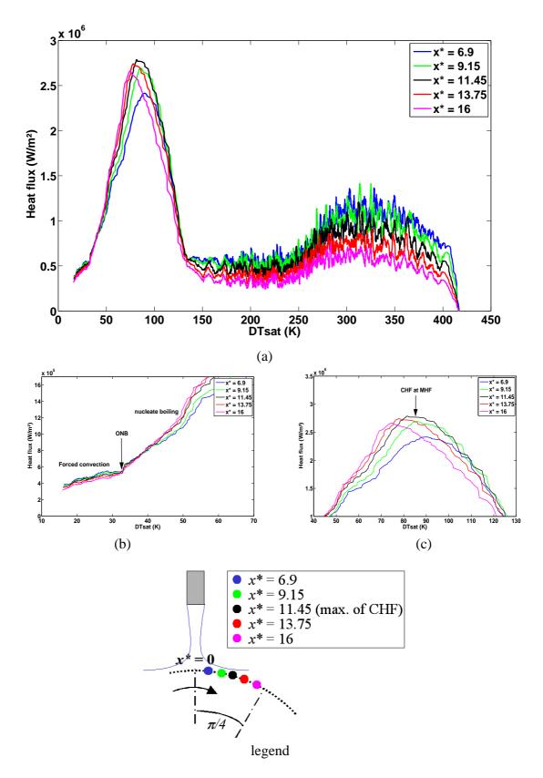
Figure 4 : local boiling curves from [16],  $\Delta T_{sub} = 34K$ ;  $u_j = 1,06 \text{ m/s} - u^* = 1,25$
