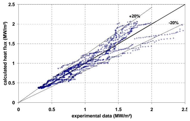
Figure 7 : Comparison between experimental data and correlation (18)
