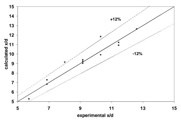
Figure 9 : Comparison between data and calculated  $x^*_{CHF,max}$  using (21)
