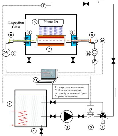
Figure 2a : Schematic of the experimental set-up [42]
