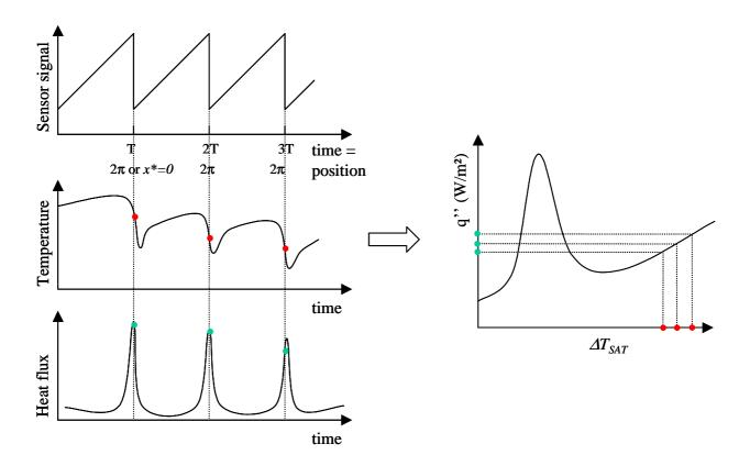
Figure 3 : Building of the boiling curves
