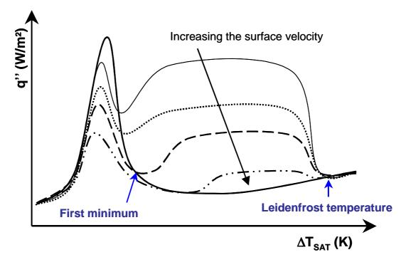
Figure 5 : shape of the local boiling curves with a moving surface
