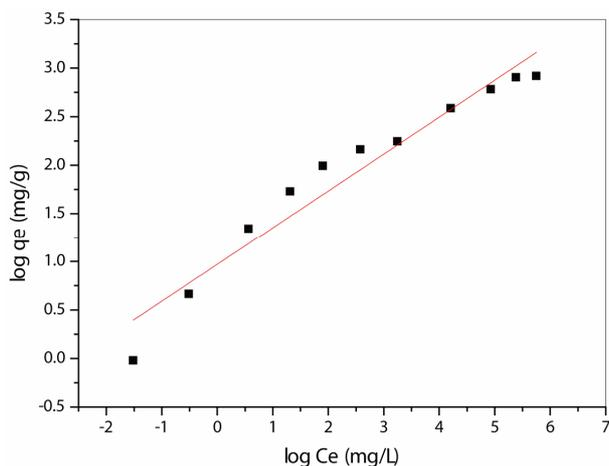
**Figure 11. Freundlich isotherm plot for adsorption of Ni<sup>2+</sup> on the maghnite.  $T = 293$  K, initial pH 7.5,  $m/V = 10$  g/L.**
