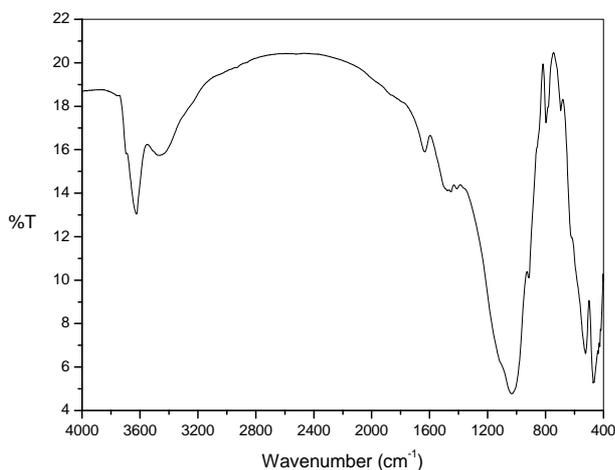
Figure 1. Infrared (IR) spectra of natural maghnite.
