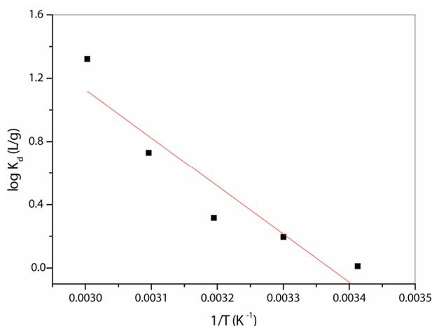
**Figure 13. Plot of  $\ln K_d$  against  $1/T$  for the adsorption of Ni(II) on maghnite, with  $R^2 = 0.895$ : For this value of  $R^2$  with four temperature value, the results are quite good compared with the literature.**
