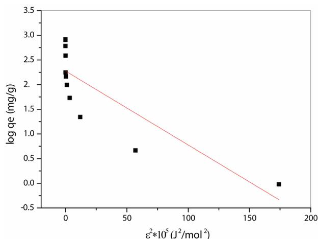
**Figure 12. D-R isotherm plot for adsorption of Ni<sup>2+</sup> on the maghnite.  $T = 293$  K, initial pH 7.5,  $m = 10$  g/L with  $R^2 = 0.664$ : To demonstrate that this type of adsorption is bad compared the two other.**
