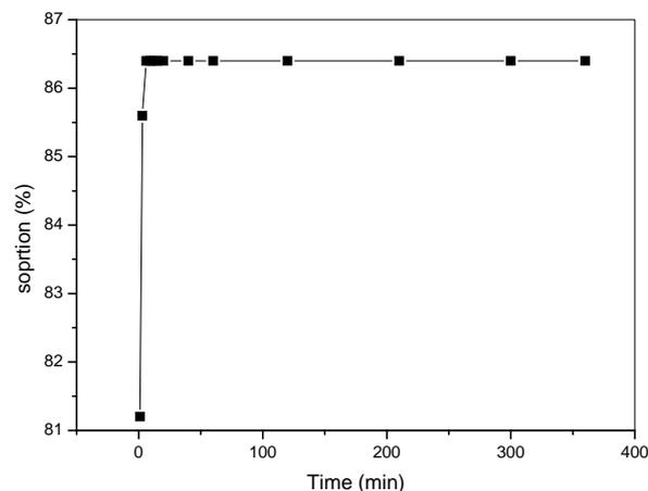
Figure 8. Effect of contact time on the adsorption of Ni(II) to maghnite, pH = 7.5 ± 0.1, T = 293 K, clay 10 g/L, C[Ni(II)]initial = 100 mg/L.
