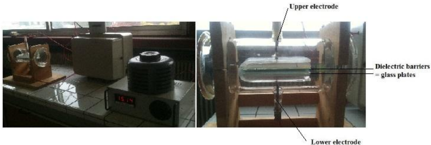
Figure 2. Corona treatment cell.
