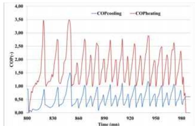
Figure 6 COP of the refrigeration adsorption machine
