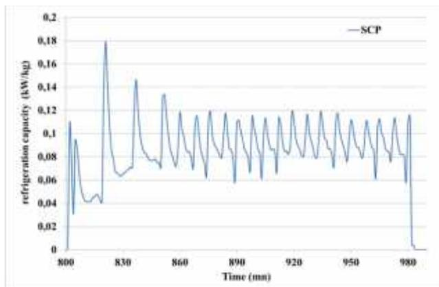
Figure 7 SCP of the refrigeration adsorption machine
