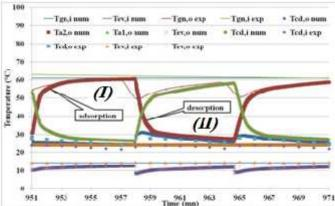
Figure 10 Temperatures profiles at the adsorbers, condenser, and evaporator (experimental and numerical)
