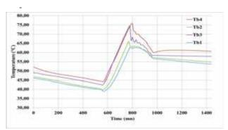
Figure 2 Evolution of the temperatures at four levels of the stratification tank
