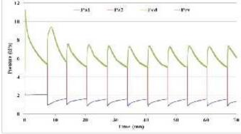
Figure 11 Pressure dynamic behavior at the adsorbers, condenser, and evaporator (numerical values)
