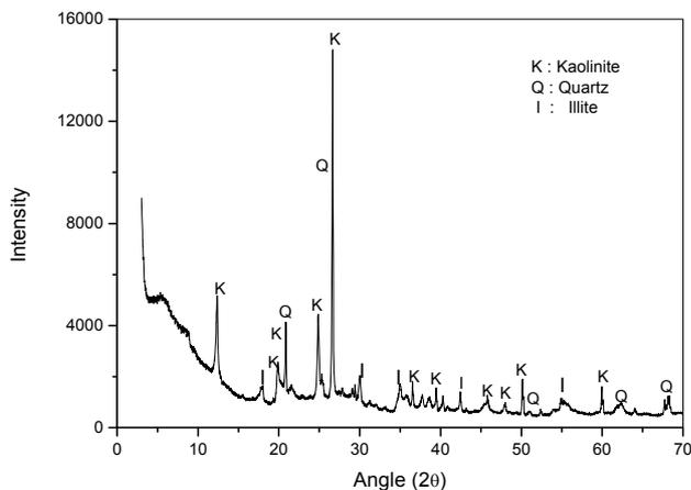
**Figure 2.** XRD pattern of kaolin.
