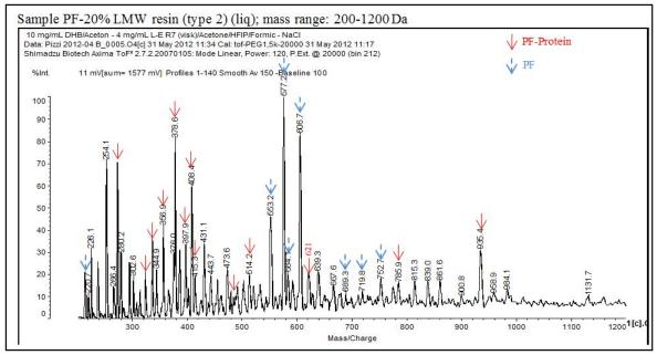
Fia. 2. MALDI-TOF spectrum of the liquid resin PF-20% LMW (type 2) for a range from 200 to 1200 Da.
