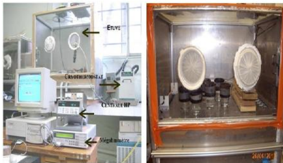
Fig. 1. Equipment and dryer at the controlled atmosphere
