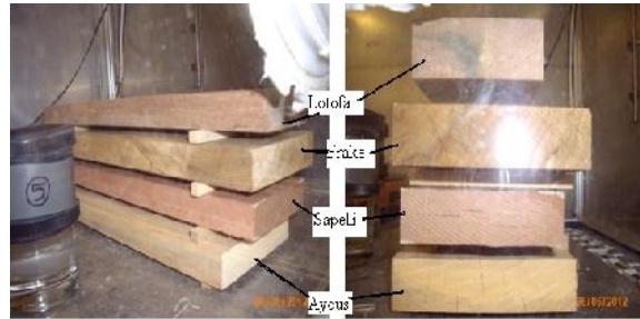
Fig. 2. Disposition of the board during the study of the drying kinetic with constant atmosphere
