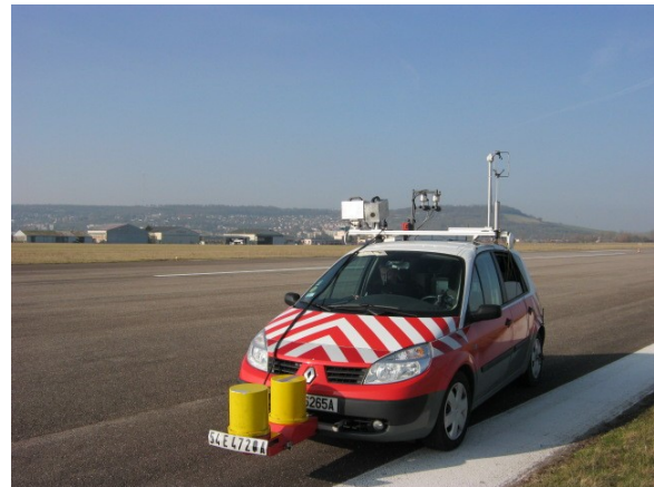
Figure 2: Instrumented vehicle used for mobile measurements within Local Climate Zones
