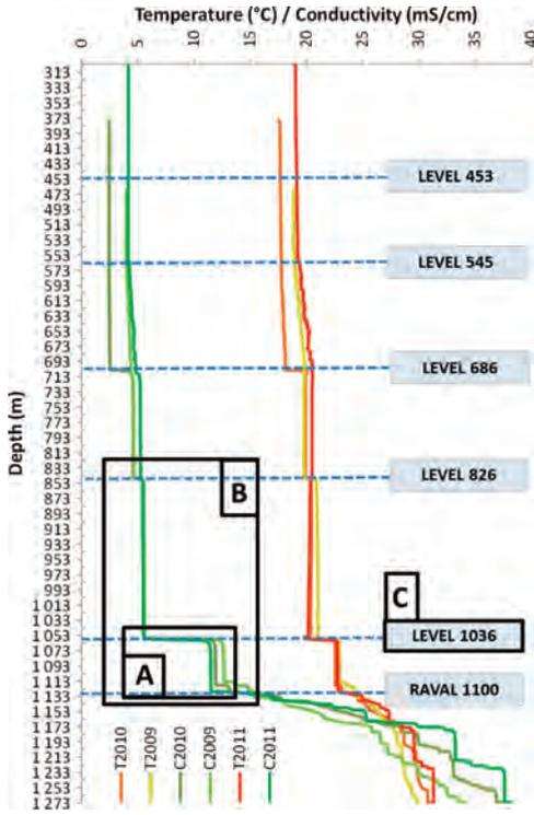
**Figure 2** Electrical conductivity (on the left) and temperature profiles (on the right) in Vouters 2 well for years 2009, 2010 and 2011 (A: Well-mixed layer capped by a step – B: thermohaline staircase – C: step corresponding to a gallery entrance).
