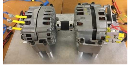
Fig. 1. Experimental test bench with two synchronous claw-pole machine
