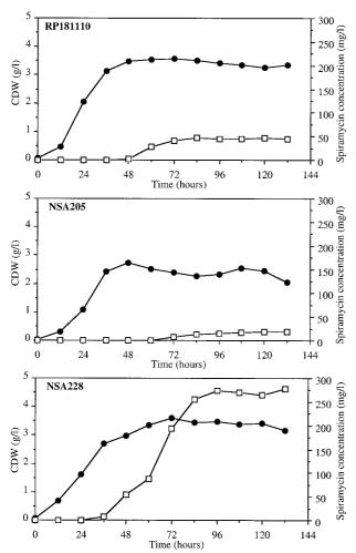
FIG. 2. Growth (●) and spiramycin production (□) of *S. ambofaciens* RP181110, NSA205, and NSA228 on a chemically defined medium in a 3-liter batch fermentor. Results are means of three independent experiments with standard deviations of 20 to 30%.
