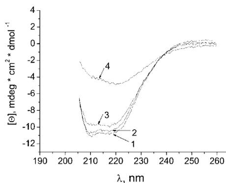
FIG. 4. Circular dichroism spectra of wild-type GAPN. (0.1 mg/ml) recorded at 25  $^{\circ}\text{C}$  in 10 mM (curves 1 and 3) and 500 mM (curves 2 and 4) potassium  $P_i$  buffer, pH 8.2, before (curves 1 and 2) and after (curves 3 and 4) 20 min of incubation at 55  $^{\circ}\text{C}$ . The samples were desalted from the stock suspension in saturated ammonium sulfate into the appropriate buffer by gel filtration prior to the experiment.
