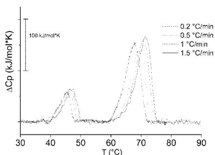
FIG. 3. Effect of the scanning rate on the thermograms of wild-type GAPN. Thermograms were recorded in 50 mM potassium  $P_i$ , pH 8.2, at a scan rate of 1.5 (solid line), 1 (dashed line), 0.5 (dotted line) and 0.2 (dashed/dotted line)  $^{\circ}\text{C}/\text{min}$ . The enzyme was dialyzed from the ammonium sulfate stock suspension in 50 mM potassium  $P_i$ , pH 6.4, for at least 20 h in the buffer before the experiment. The protein concentration was 0.2 mg/ml.  $T$ , temperature.
