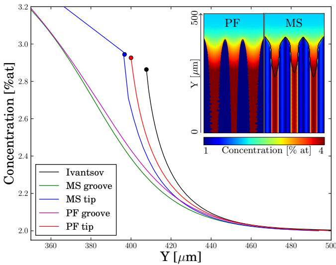
**Fig. 2.** Liquid concentration profiles along the axis of a primary arm and along a groove between two arms. Comparison of a phase-field and a mesoscopic simulation at the steady state ( $t = 50 \text{ s}$ ). The Ivantsov solution for a free tip growing at the pulling speed is also shown for comparison. The inset shows the full concentration fields from the phase-field (PF) and mesoscopic (MS) simulations.
