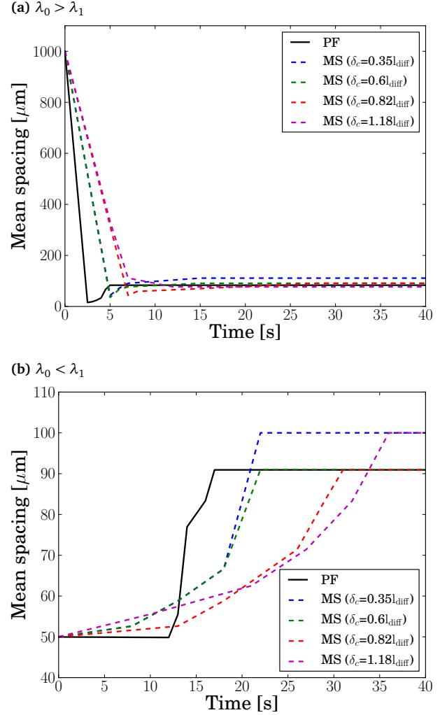
**Fig. 7.** Evolution of the average primary arm spacing in the phase-field and mesoscopic simulations for two initial spacings,  $\lambda_0$ . (a)  $\lambda_0 = 1000 \mu\text{m}$ , (b)  $\lambda_0 = 50 \mu\text{m}$ . The results of the mesoscopic model are from simulations with three different stagnant-film thicknesses,  $\delta_c$ .
