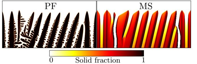
**Fig. 11.** Dendrite structure given by the phase-field (PF) and by the mesoscopic model (MS) for  $\alpha_0 = 20^\circ$  at  $t = 20$  s.
