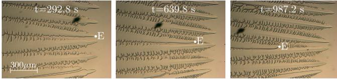
**Fig. 4.** Mechanisms of primary spacing adjustment. Micrographs of directional solidification of an NPG-TRIS (neopentyl glycoltris(hydroxymethyl)aminomethane) alloy, courtesy of Victor Witusiewicz (Access e.V).
