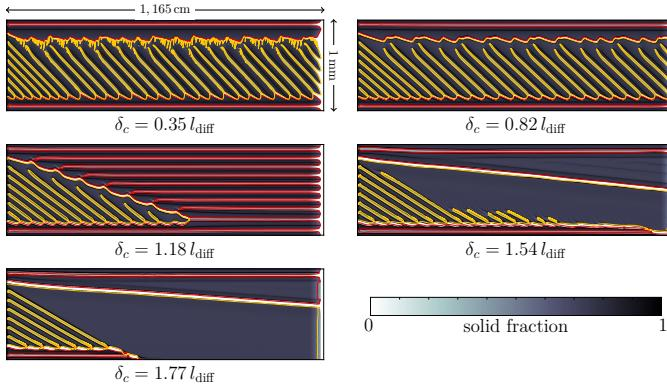
Fig. 15. The influence of the stagnant-film thickness,  $\delta_c$ , on the growth competition between the well oriented (red contour) and the misoriented (yellow contour) grains ( $\alpha_0 = 20^\circ$ ,  $t = 200$  s, solid fraction is superimposed). Note that the horizontal length is displayed compressed by a factor of 0.3.
