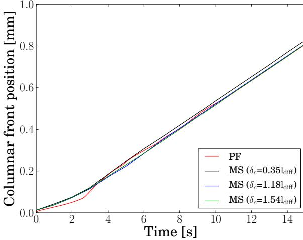
**Fig. 6.** Evolution of the columnar front position in the phase-field (PF) and mesoscopic (MS) simulations for  $\lambda_0 = 1000 \mu\text{m}$ . The results for  $\lambda_0 = 50 \mu\text{m}$  are similar and are not shown to avoid overlap. The results of the mesoscopic model are from simulations with three different stagnant-film thicknesses,  $\delta_c$ .
