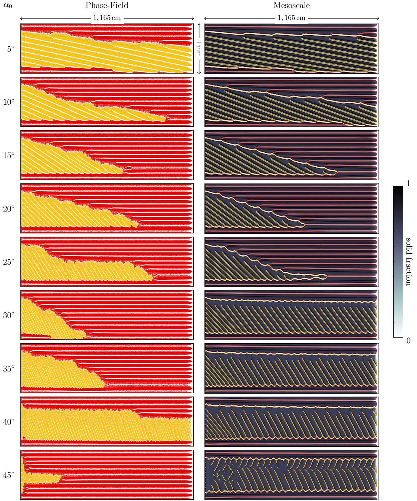
**Fig. 12.** Spatiotemporal plots of growth competition predicted by the phase-field (left) and the mesoscopic model (right). The well-oriented grains are shown in red and the grain misoriented by the angle  $\alpha_0$  is shown in yellow (full for phase field, contour for mesoscale where solid fraction is superimposed). Note that the horizontal length is displayed compressed by a factor of 0.3.
