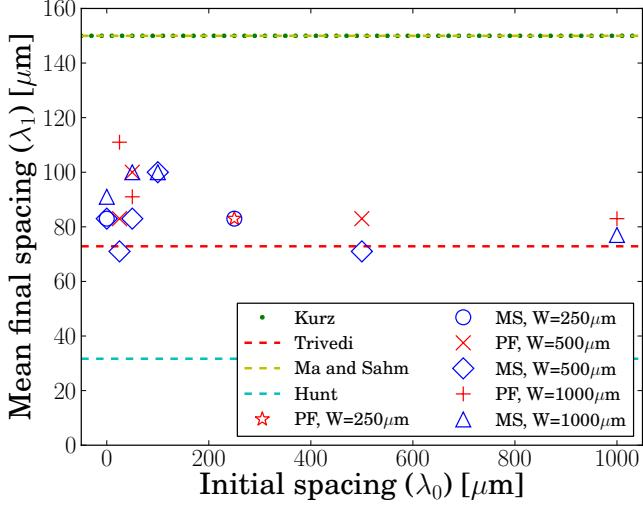
**Fig. 8.** Dependence of the final primary arm spacing on the spacing of the initial nuclei,  $\lambda_0$ , and on the width of the confinement  $W$ . Mesoscopic simulations with an initially planar front are characterized by an initial spacing of  $\lambda_0 = 0$ . All MS results are from simulations with  $\delta_c = 1.18 l_{\text{diff}}$ .
