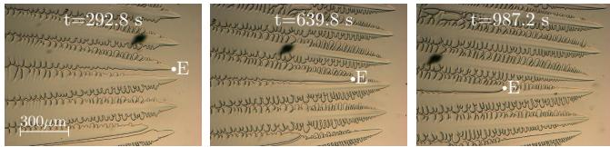
**Fig. 4.** Mechanisms of primary spacing adjustment. Micrographs of directional solidification of an NPG-TRIS (neopentyl glycol-tris(hydroxymethyl)aminomethane) alloy, courtesy of Victor Witusiewicz (Access e.V.).
