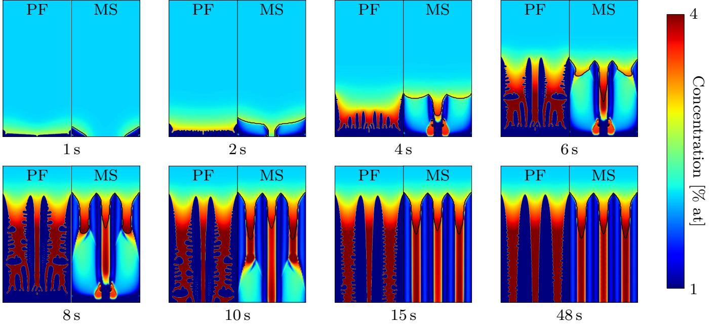
**Fig. 1.** The evolution of the columnar grains during directional solidification initiated from two nuclei placed in the bottom corners. Fields of average concentration calculated by phase field (PF, left) and by the mesoscopic (MS, right) model. The envelope of the mesoscopic model is shown as a black line. The domain width is  $250 \mu\text{m}$ .
