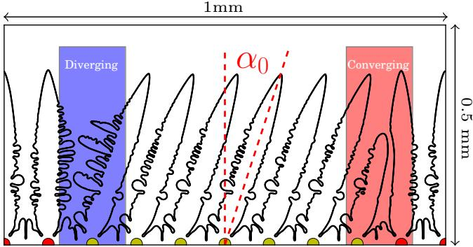
**Fig. 10.** Schematics of the calculation domain and of the initial conditions. The semicircles represent the initial seeds and their crystal orientations: yellow and red for the misoriented and the well-oriented grains, respectively.
