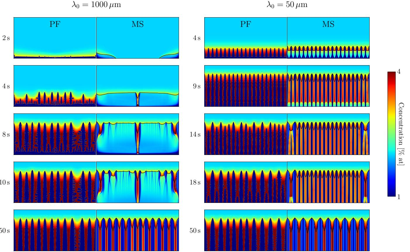
**Fig. 5.** The evolution of the columnar grains from an initial spacing of  $\lambda_0 = 1000 \mu\text{m}$  (left column) and  $\lambda_0 = 50 \mu\text{m}$  (right column). The domain size is  $500 \times 1000 \mu\text{m}$ . The concentration field is shown for phase field (PF) and the average concentration field and the envelope (black line) are shown for the mesoscopic model (MS).
