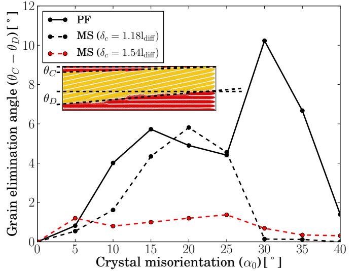
Fig. 13. Grain elimination angles as function of the crystal misorientation angle  $\alpha_0$  of the misoriented grain. Comparison between mesoscopic (MS) simulations for two stagnant-film thicknesses and the phase-field (PF) simulations. Grain elimination angles for smaller stagnant-film thicknesses ( $\delta_c < 1.18 l_{\text{diff}}$ ) in the MS model were zero.
