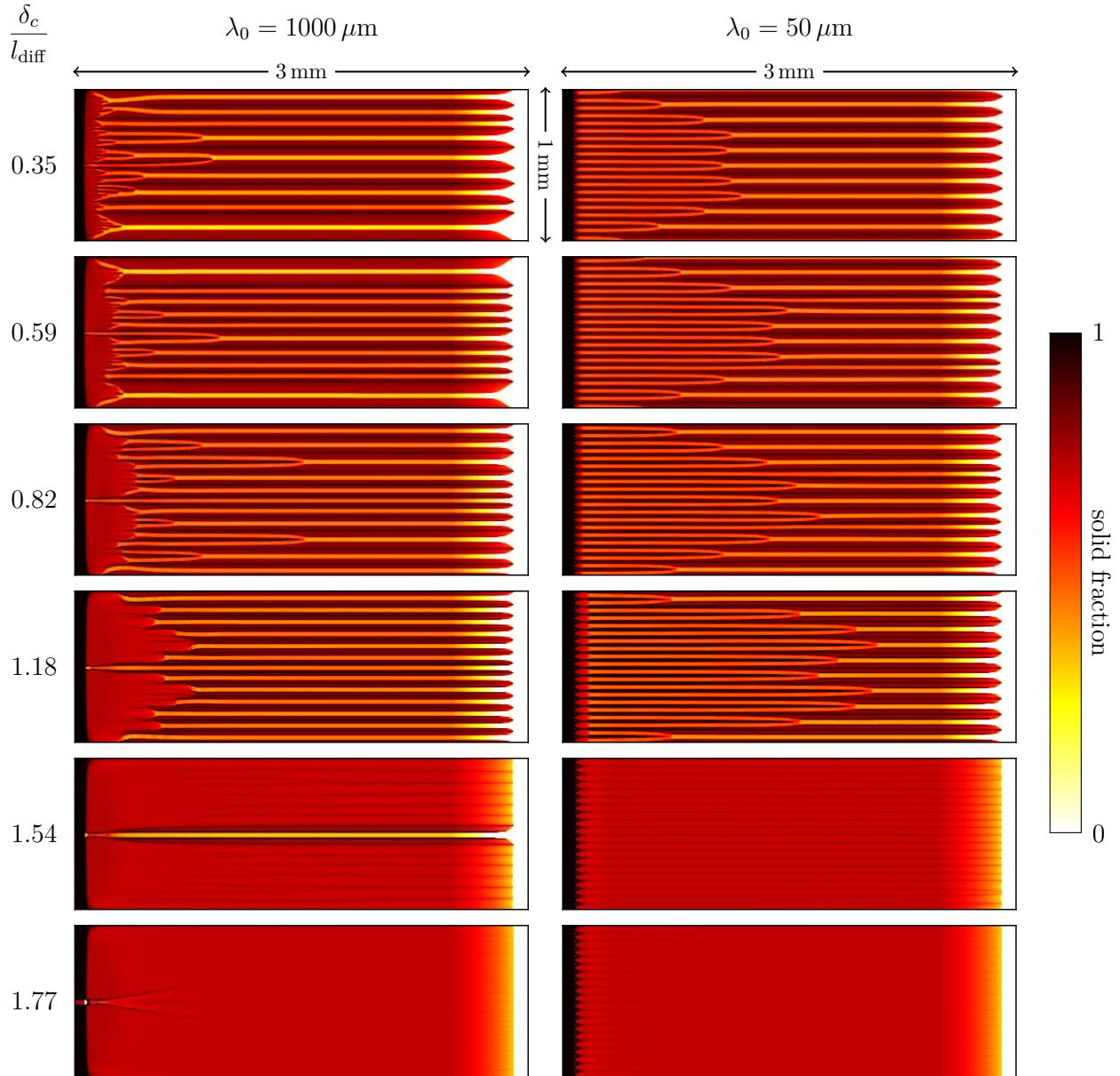
**Fig. 9.** Spatiotemporal plots of mesoscopic simulations with different stagnant-film thicknesses,  $\delta_c$ . The plots show the solid fraction and were reconstructed from the moving-frame simulations up to  $t = 50\text{s}$ .
