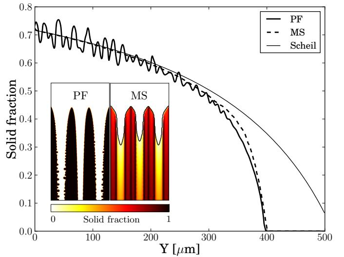
**Fig. 3.** Average solid-fraction profiles along the height of the mushy zone for phase field (PF) and mesoscopic (MS) simulations, and for the Scheil model. The inset shows the full solid fraction fields from both simulations.
