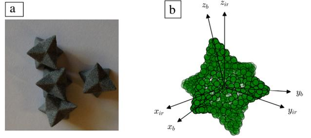
**Figure 1.** a) Experimental model equiaxed dendritic grain envelope ( $\theta = 45^\circ$ ,  $d_{eq} = 7 \text{ mm}$ ) and b) numerical equiaxed dendritic grain envelope ( $\theta = 45^\circ$ ,  $d_{eq} = 7 \text{ mm}$ ). The surface is described with 527 spherical elements ( $l_c/d_{sph} \approx 20$ ). The indexes  $ir$  and  $b$  refer to inertial reference and body frames, respectively.
