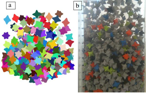
**Figure 2.** Random packing of equiaxed dendritic grain envelope ( $\theta = 45^\circ$ ,  $d_{eq} = 7 \text{ mm}$ ): a) DEM simulation, b) Experimental validation packing.
